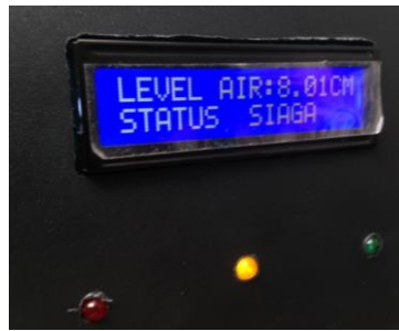
Figure 13. Test results on "SIAGA" status.
