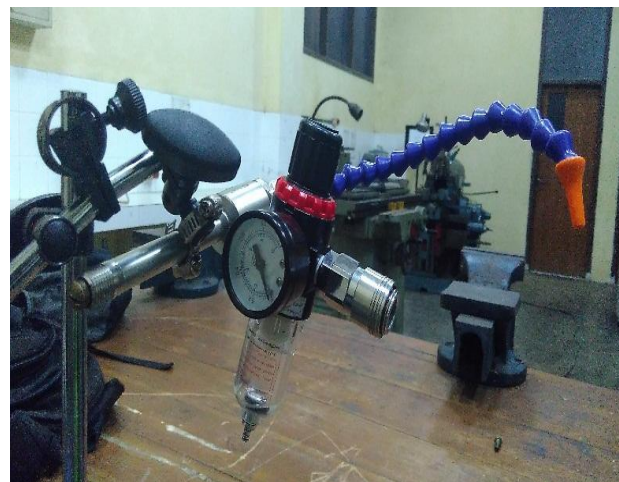
Figure 2. Vortex tube used to produce air cooling.
