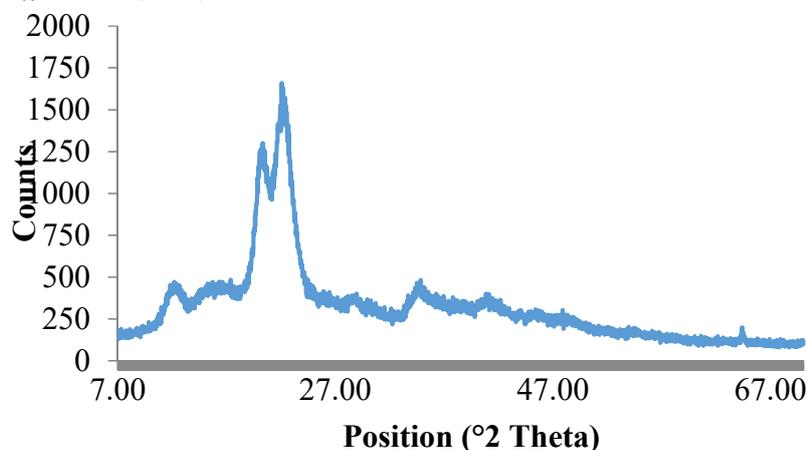
**Figure 1.** X-Ray Diffraction Graph of Microcrystalline Cellulose from Cocoa Pod Husk
