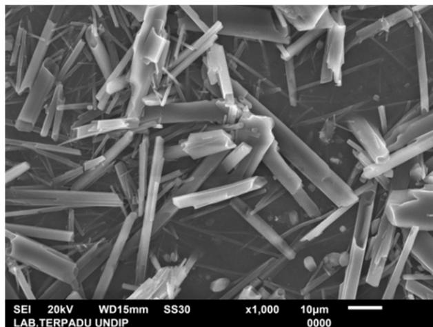
**Figure 2.** Microcrystalline cellulose with magnification 1000x
