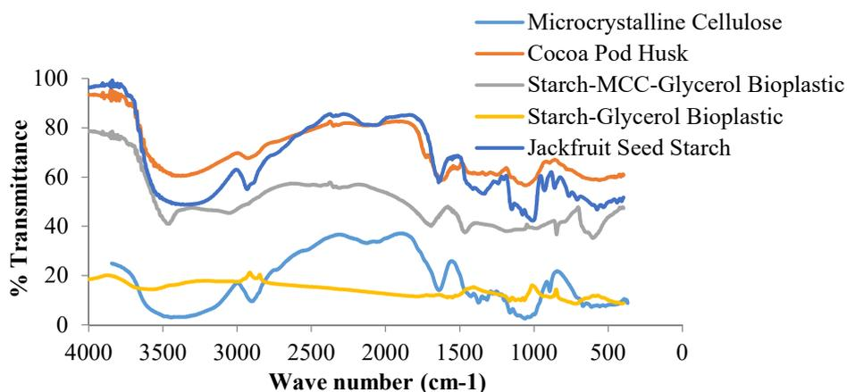
**Figure 5.** Characteristics of FT-IR spectra analysis
