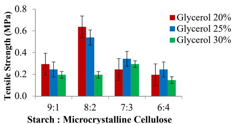
**Figure 3.** The effect of microcrystalline cellulose and glycerol addition on tensile strength of bioplastic from jackfruit seed starch
