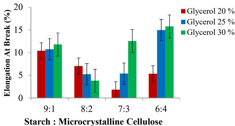
**Figure 4.** The effect of microcrystalline cellulose and glycerol addition on elongation at break of bioplastic from jackfruit seed starch
