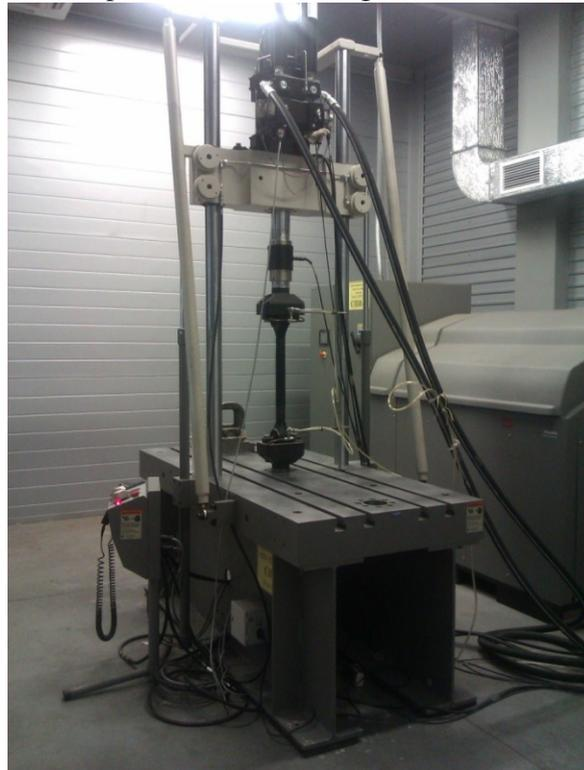
**Figure 1.** Test bench with installed steering traction during the test.
