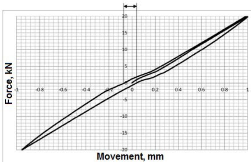
**Figure 5.** Example of the load diagram for the test for determining the gap in the friction pair "Ball pin – body of the tie-rod end".
