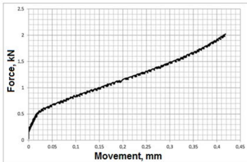
**Figure 3.** Example of the loading diagram in the test for determining the magnitude of the axial displacement and the force of compression.
