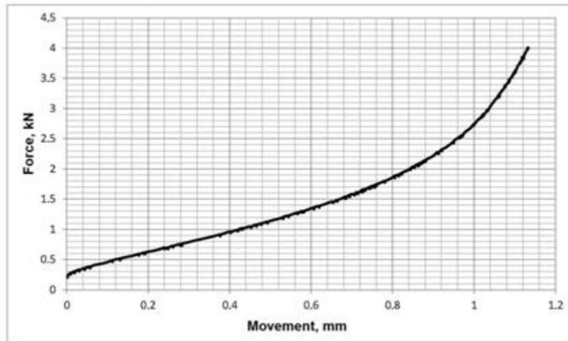
**Figure 6.** Example of the loading diagram in the test for determining the magnitude of the axial displacement and the force of the pinching: the elastic element is not compressed, the tie-rod end is inoperable.
