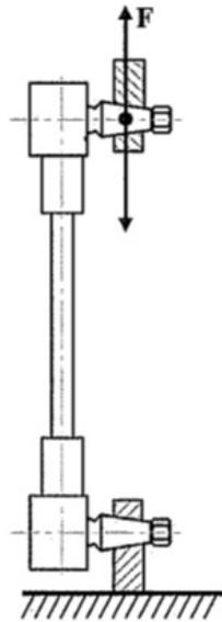
**Figure 4.** The scheme of fastening and loading of steering drafts in tests for determining the gap in the friction pair "Ball pin - body of the tie-rod end " with the radial cyclic action of the load.
