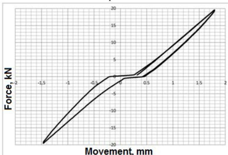
**Figure 7.** Example of the loading diagram for the gap test: a pronounced rearrangement has occurred, the tie-rod end is inoperable.
