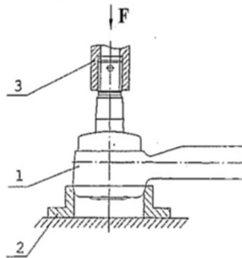
**Figure 2.** Scheme of fixing and loading the tip of the thrust during the test to determine the axial displacement and the compression force: 1 – test sample, 2 – basic rigging, 3 – transition element.
