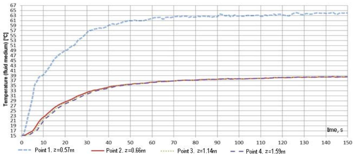
**Figure 6.** Graphs of temperature change in time in the outlet pipe at different distances from the heater with static heating. In all cases,  $x = 0.969\text{m}$ ,  $y = 0.988\text{m}$ .
