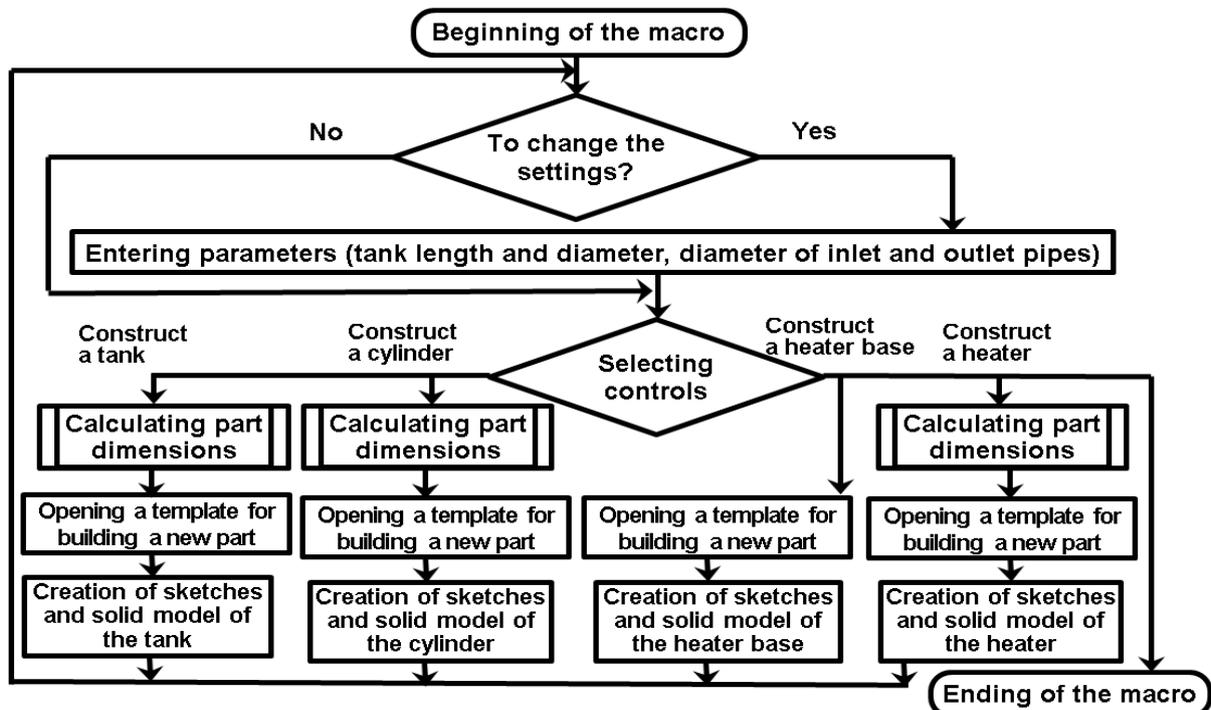
**Figure 2.** Simplified algorithm for the operation of the macro for forming the assemblies of the heating module.
