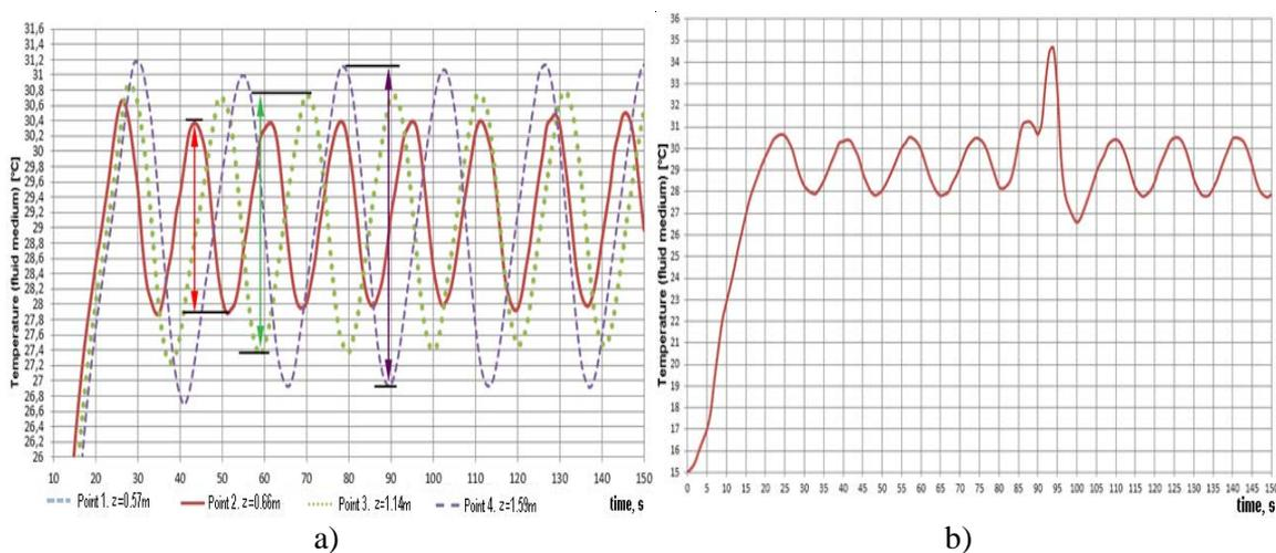
**Figure 7.** The time dependences of the temperature changes during the operation of the thermostat system in the threshold mode for different locations of the temperature sensor (a) and the transient diagram when the flow rate is changed (b). The sensor is placed in the position  $z = 0.66\text{m}$ .
