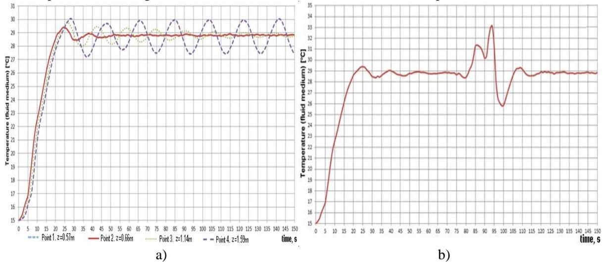
**Figure 8.** The graph of the temperature changes during the operation of the thermostat system in the proportional control mode for various locations of the temperature sensor (a) and the transient schedule when the flow rate is changed (b). The sensor is placed in position  $z = 0.66\text{m}$ .
