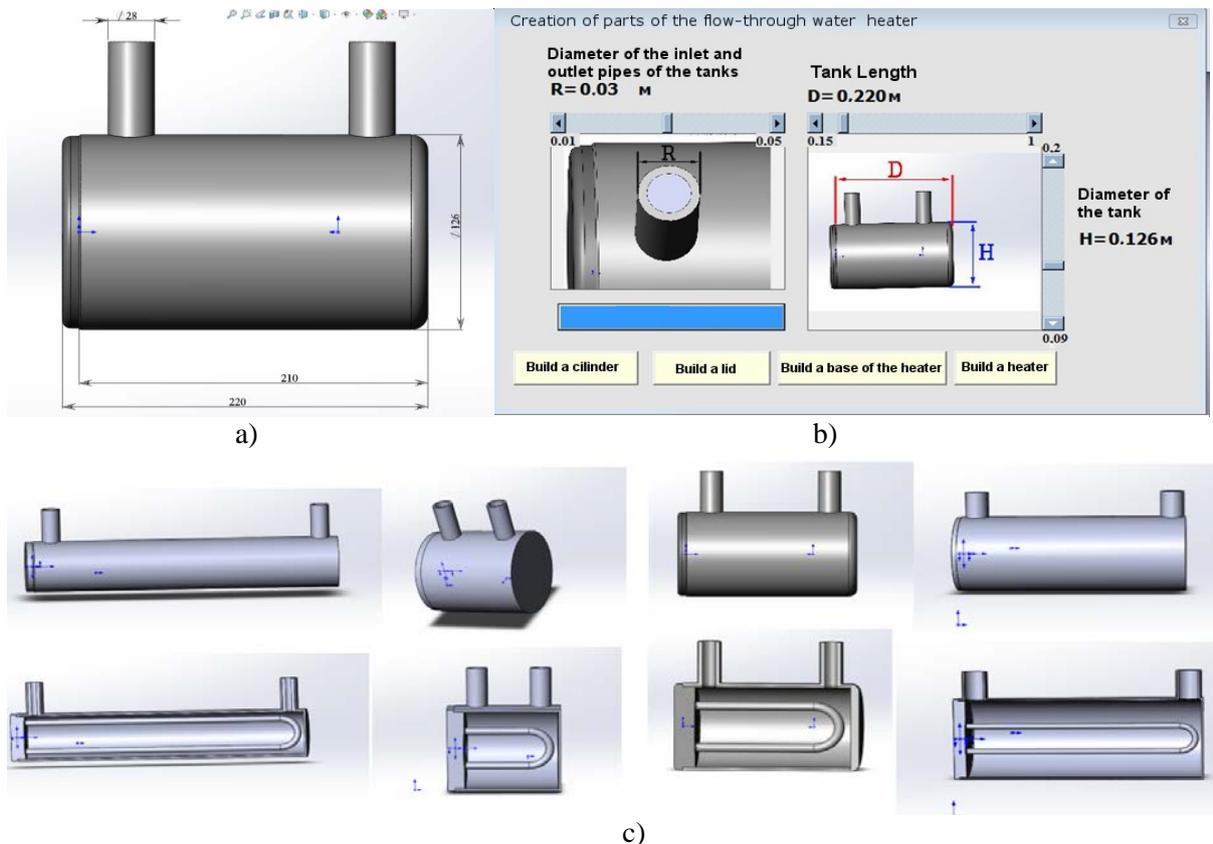
**Figure 1.** The design of the heating module (a), the dialog form of the macro for entering the parameters of its assembly (b), and the various variants of such assemblies, constructed with this macro (c).
