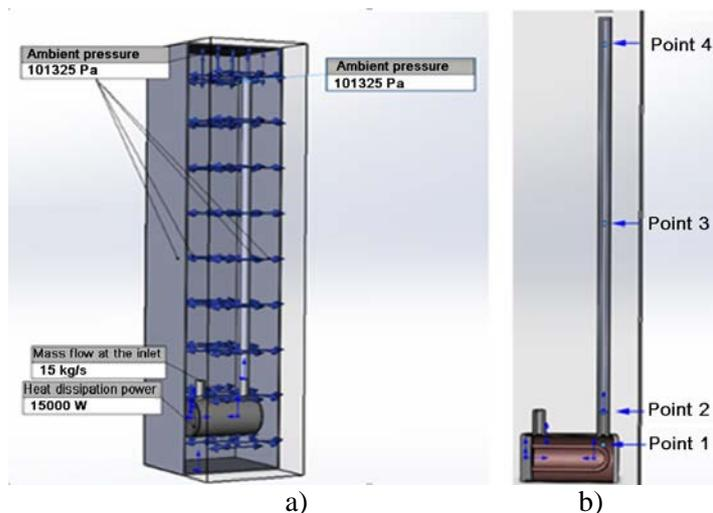
**Figure 4.** Type CAE model for the study of heat distribution in a flow-through water heater with specified boundary and initial conditions (a) and placement of points on it for monitoring the temperature of heated water (b).
