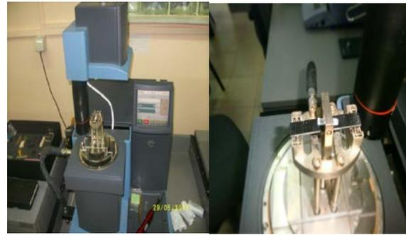
**Figure 4.** The type of the three point bending clamp used in mechanical testing in TA Q800 DMA.
