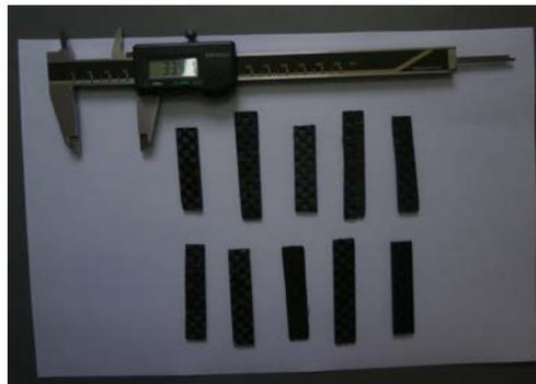
**Figure 2.** Specimens of CFRPs used for mechanical testing.
