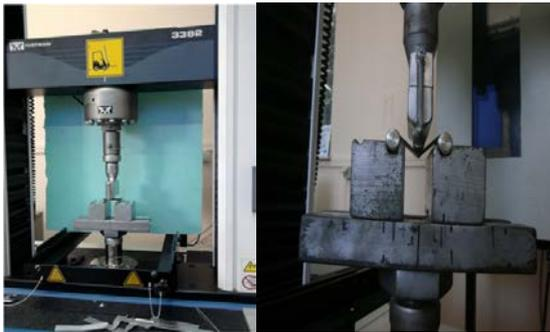
**Figure 3.** Three point bending tests procedure in Instron 3382 UTM.
