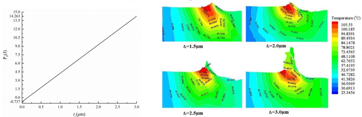
Figure 5. The total power for analysis results Figure 6. Workpiece temperature cloud at different uncut chip thickness
