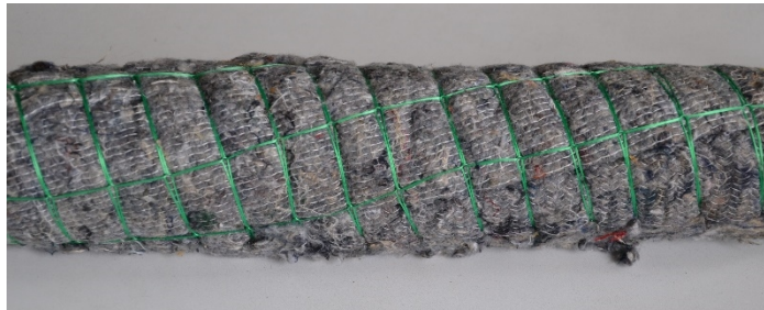
Figure 3. The Kemafil rope manufactured from the nonwoven made from blended recycled fibres.
