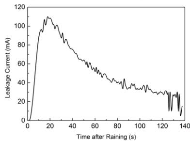
**Figure 7.** Leakage current envelope of No.1 bushing.
