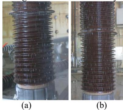
**Figure 12.** Distribution of rain curtains on bottom of No.2 bushing.
