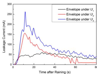
**Figure 5.** Leakage current envelope under Different Voltage.
