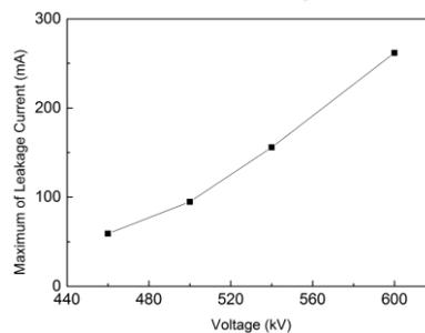
**Figure 6.** Maximum of leakage current under different voltage.
