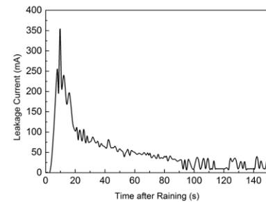
**Figure 9.** Leakage current envelope of No.3 bushing.
