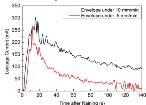
**Figure 11.** Leakage current envelope of No.2 bushing under different rainfall.
