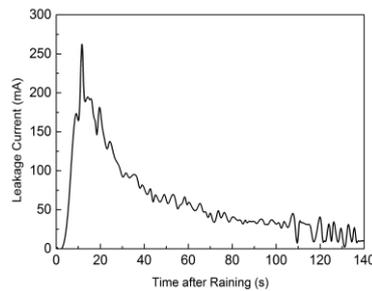
**Figure 8.** Leakage current envelope of No.2 bushing.
