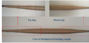
Figure 1. Structure of capacitance core.
