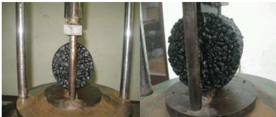
Figure 7. The setting experiment of Indirect Tensile Strength Test
