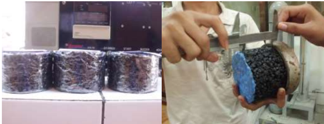
Figure 5. The sample for vertical and horizontal permeability Test
