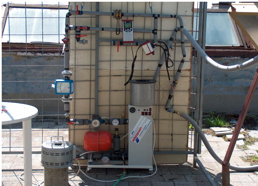
Figure 3. Picture of part of the measuring line for hydraulic and thermotechnical tests of solar thermal panel
