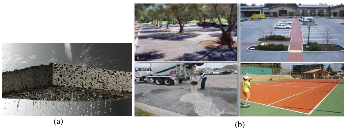
Figure 1. (a) Pervious concrete [8] and (b) Typical uses of pervious concrete [9].
