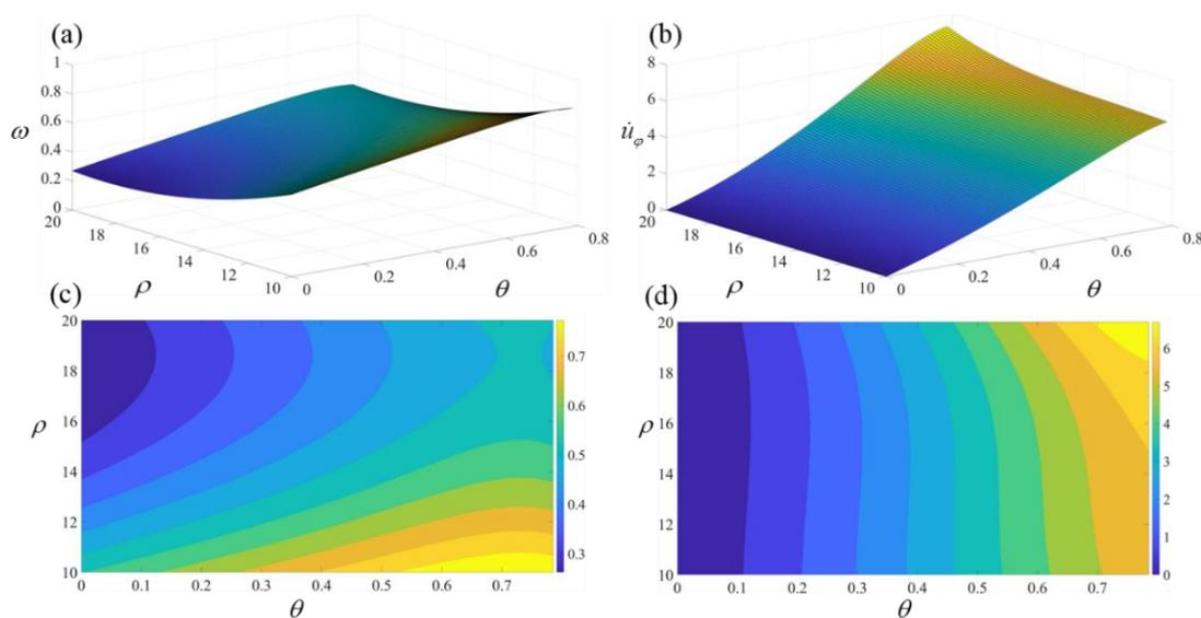
**Figure 10.** The velocity distribution of billet inside the rotating die; (a) the angular velocity; (b) the circumferential velocity; (c) the contour of angular velocity; (d) the contour of circumferential velocity.
