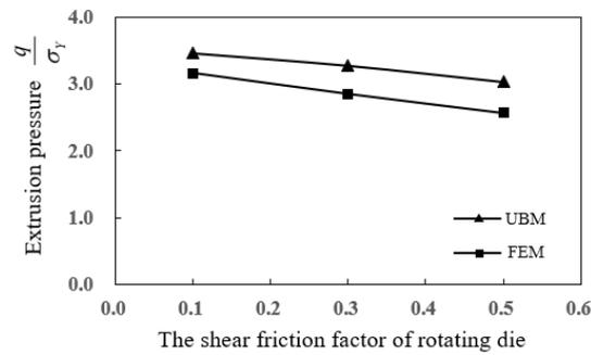
**Figure 8.** The comparison of relative extrusion force.
