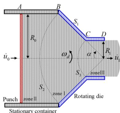
**Figure 1.** Schematic representation of TE process.
