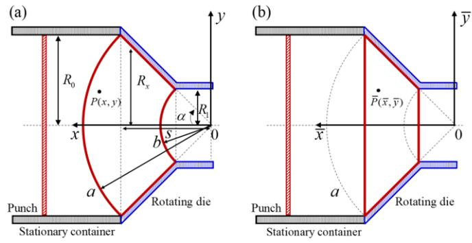
**Figure 4.** The schematic diagram of mapping relation; (a) deformation zone; (b) mapping zone.
