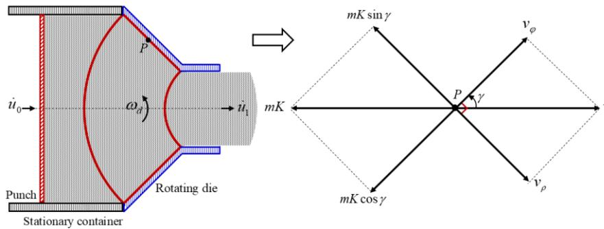
**Figure 6.** Shear stress distribution of the billet on the outer surface of the point.
