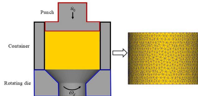
**Figure 7.** The finite element model.
