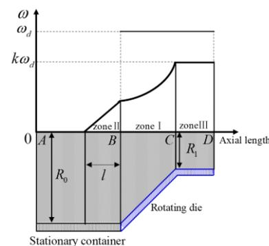
**Figure 2.** The distribution of rotating angular velocity of billet at the outside surface.
