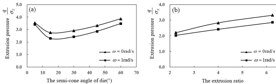
**Figure 9.** The variation of relative extrusion force; (a) the semi-cone angle of die; (b) the extrusion ratio.
