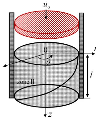
**Figure 5.** Deformation of billet inside the container
