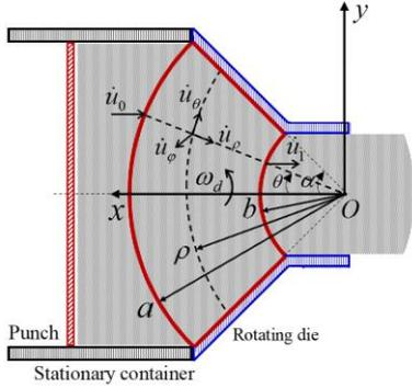
**Figure 3.** Compound spherical velocity field.
