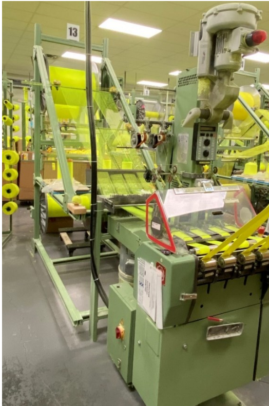
Figure 1. Narrow width loom at DTS.
