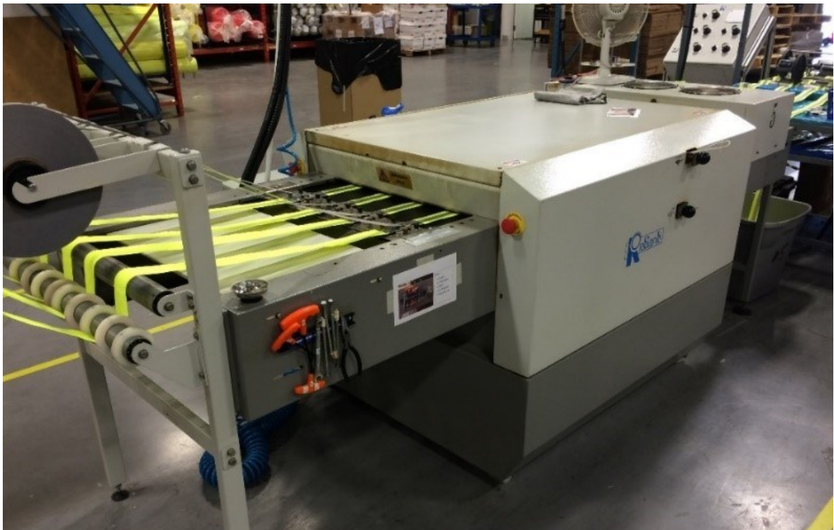
Figure 3. Narrow fabric and reflective trim entering the fusing machine at DTS.
