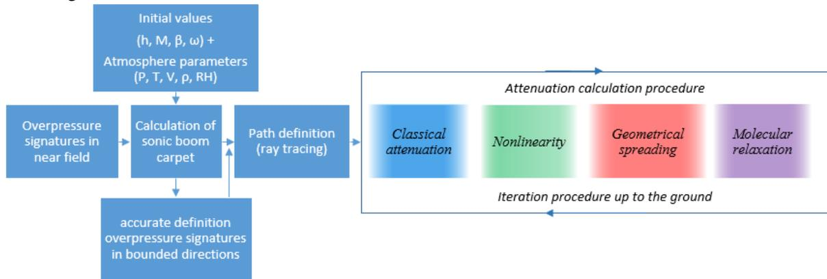
**Figure 2. Procedure for calculating the propagation and attenuation of a sonic boom**
