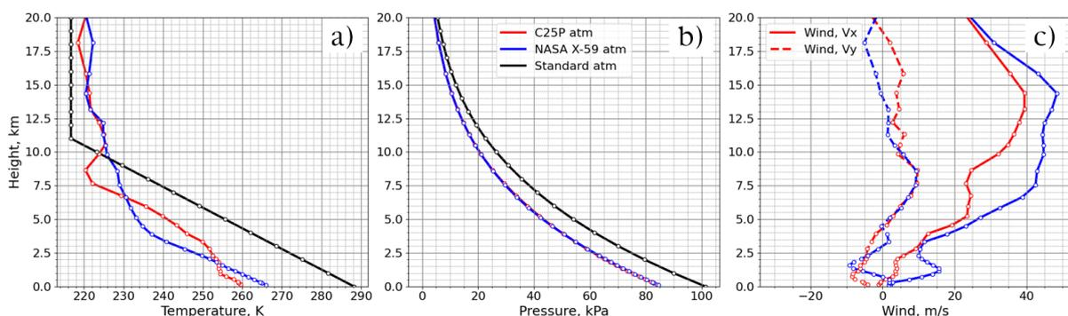
**Figure 3. Atmosphere temperature (a), pressure (b) and winds profiles (c)**
