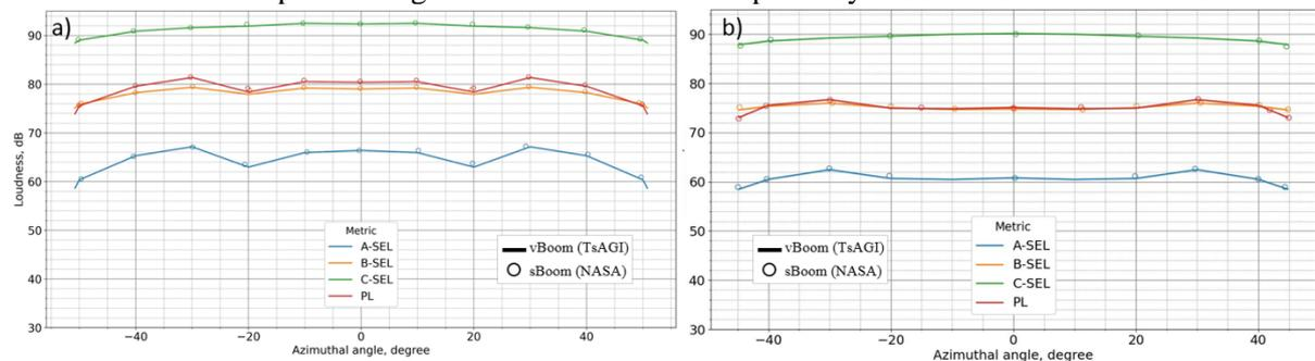
**Figure 6.** Loudness in different metrics (A-SEL, B-SEL, C-SEL, PL) for C25P (a), and NASA X-59 (b) during propagation in condition of standard atmosphere without wind
