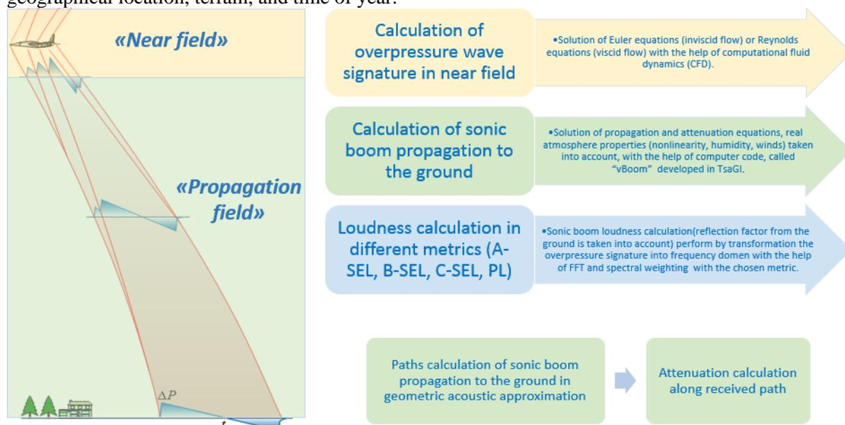
**Figure 1.** Procedure to evaluate characteristics of sonic boom on the ground.
