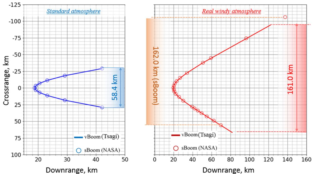
**Figure 8.** Sonic boom carpet at the ground for NASA X-59 during propagation in condition of standard without wind (a) and real windy atmosphere (b)
