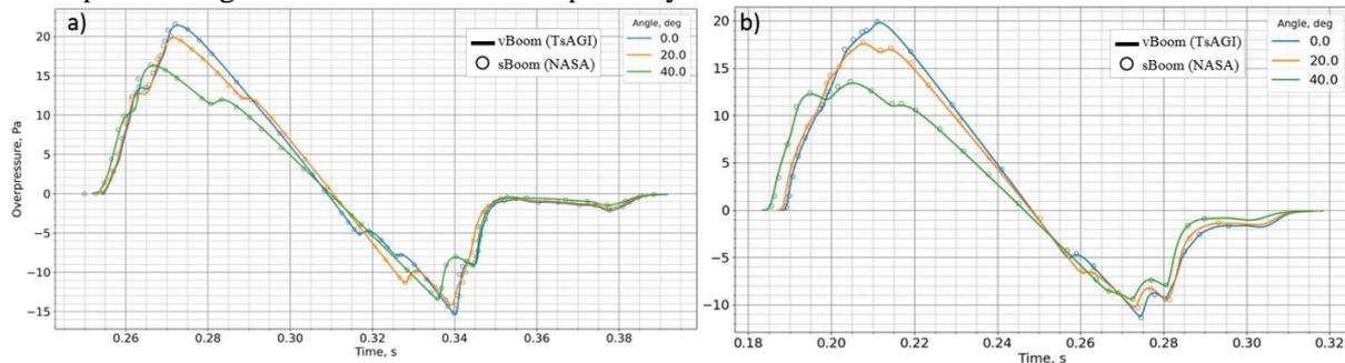
**Figure 4.** Overpressure signatures at the ground for C25P (a), and NASA X-59 (b) during propagation in condition of standard atmosphere without wind
