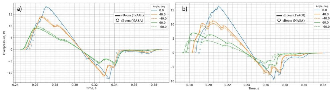
**Figure 5.** Overpressure signatures at the ground for C25P (a), and NASA X-59 (b) during propagation in condition of real windy atmosphere
