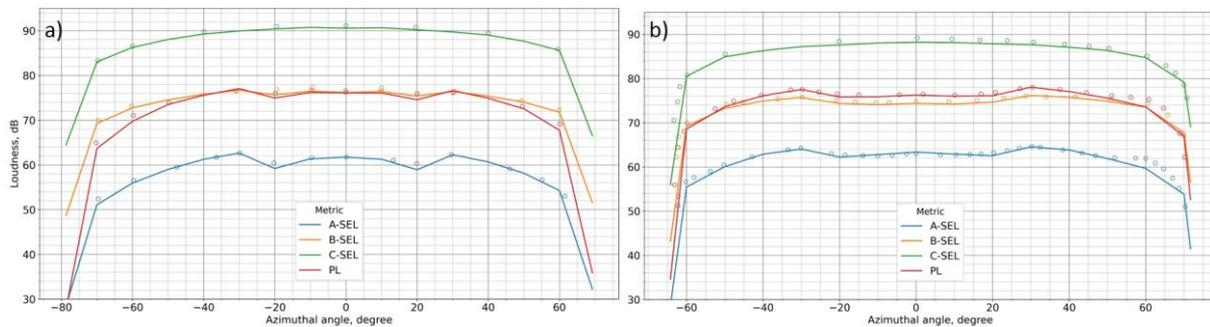
**Figure 7.** Loudness in different metrics (A-SEL, B-SEL, C-SEL, PL) for C25P (a), and NASA X-59 (b) during propagation in condition of real windy atmosphere
