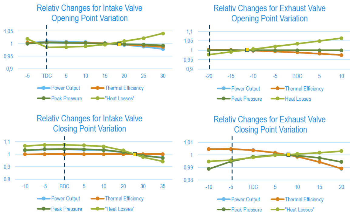
Figure 6: Relative changes in piston engine key parameters for valve timing variation
