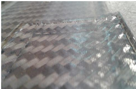
Figure 7 – Tooling mark off on the part
