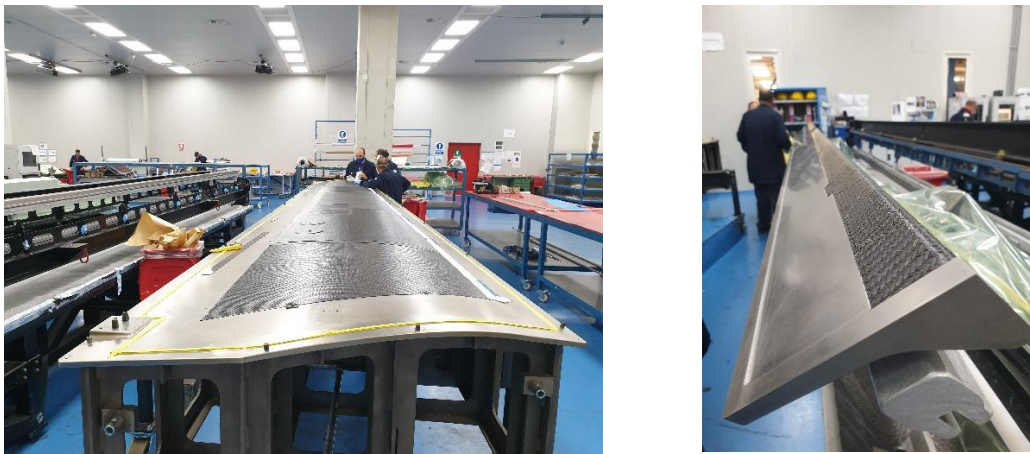
Figure 2 - Hand layup in clean room – skin tool mold and mandrel
