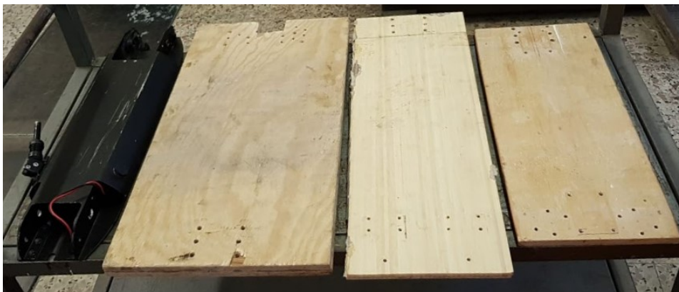
Figure 2. Decks A 2 , E, B, C (from left to right); deck E has been discarded from subsequent tests, because of high similarity with deck A 2 in terms of stiffness.
