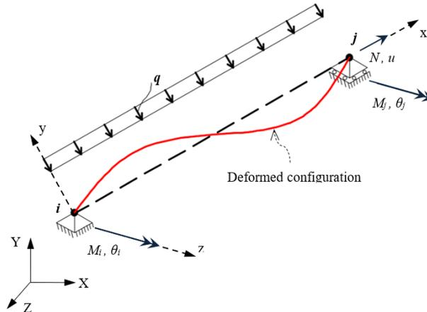
**Figure 3.** Beam-Column element with rigid-body modes removed.
