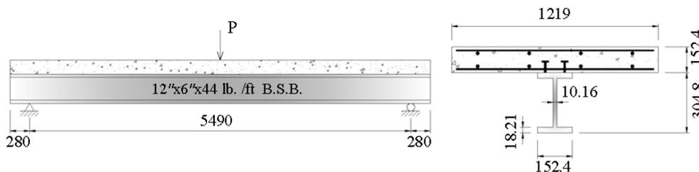
Figure 4. Beam E1 layout
