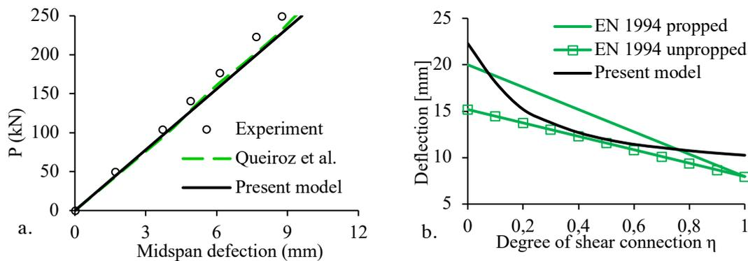
**Figure 5.** a. Load-deflection curves; b. Deflection-shear connection degree curves.
