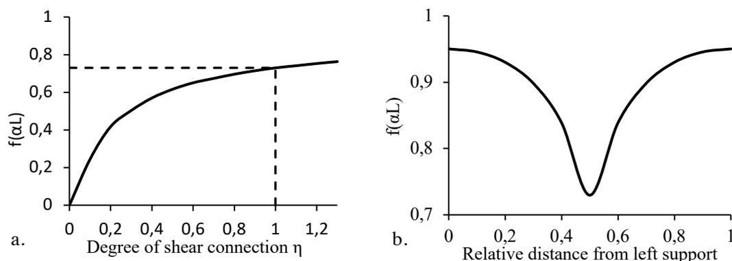
**Figure 6.** a.  $f(\alpha L)$ -degree of shear connection curve; b.  $f(\alpha L)$  variation along the beam length
