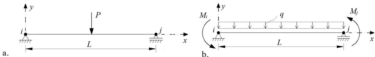
**Figure 2.** **a.** Simply supported beam subjected to concentrated load; **b.** Simply supported beam subjected to end bending moments and uniform distributed load.
