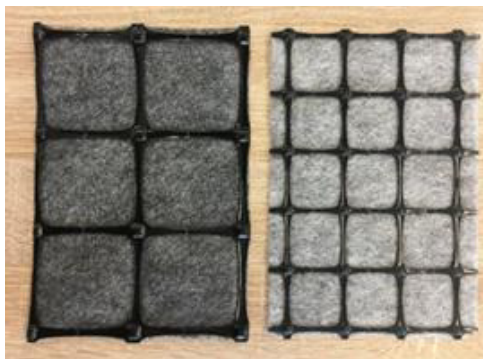
Figure 6. Geocomposites incorporating biaxial grids. Large version of 65x65 mm (left) and small version of 39x39 mm aperture size (right)
