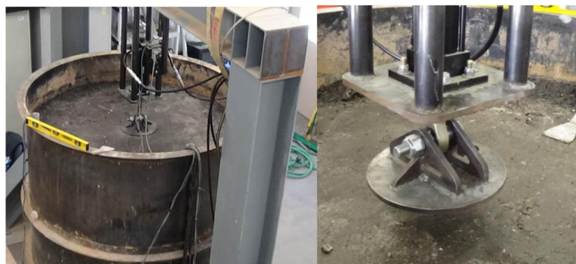
Figure 2. Tank and steel loading plate used in Nevada DOT test
