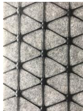
Figure 7. Geocomposite incorporating triaxial grid with the hexagonal pitch of nominal value of 80 mm
