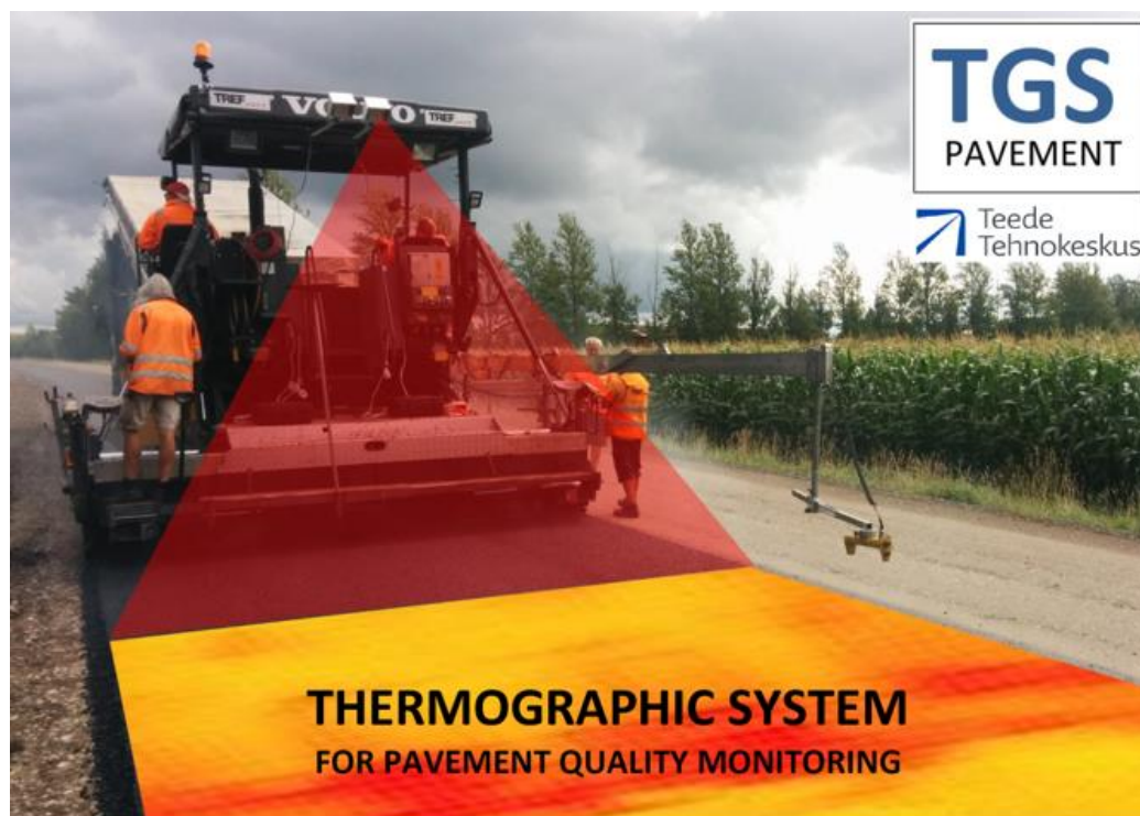
Figure 1. TGS Pavement thermographic system attached to paver.
