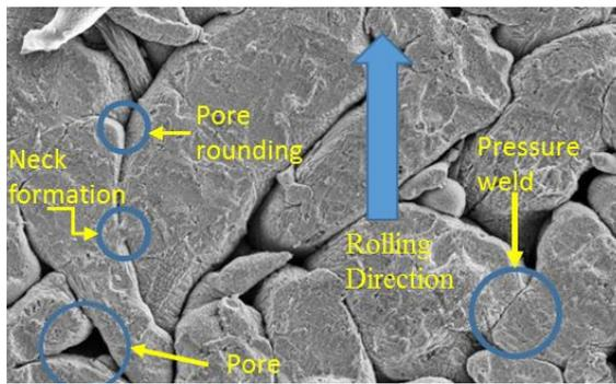
**Figure 8.** SEM-SE image of an aluminium strip surface after being rolled at 0.7 mm and sintered at 580 °C.
