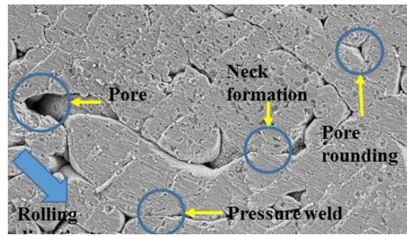
**Figure 12.** SEM-SE image of an aluminium strip surface after being rolled at 0.75 mm and sintered at 580 °C, then re-rolled at 0.7 mm roll gap then re-sintered at 580 °C.
