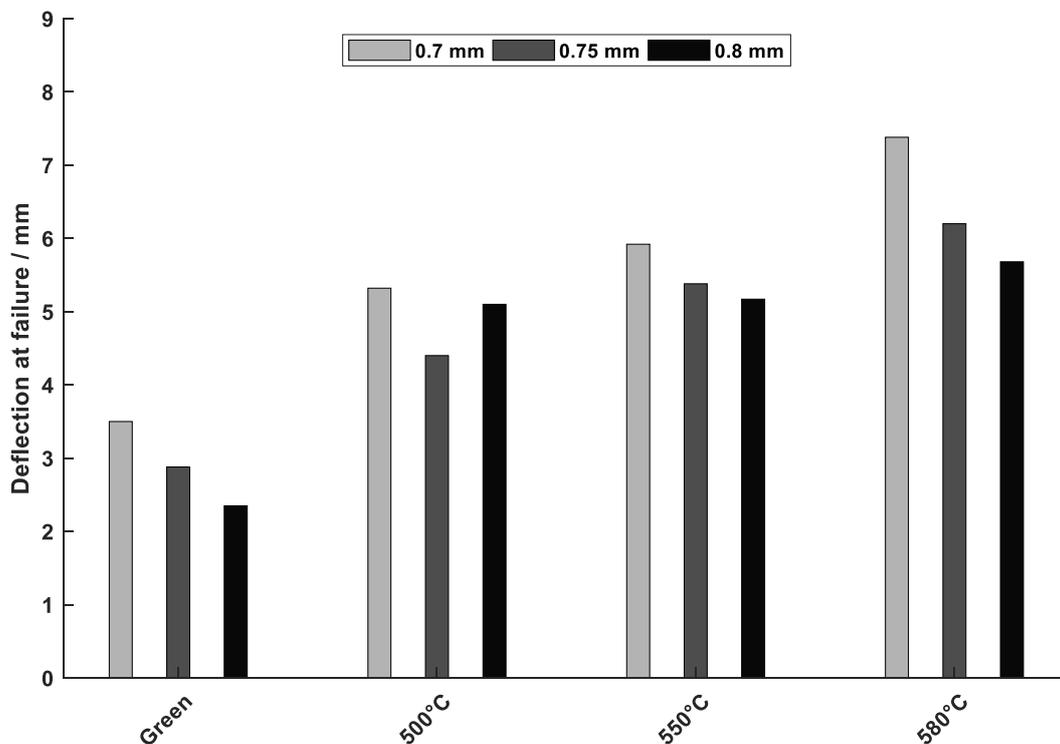
**Figure 14.** Bar graph representing aluminium strip maximum deflection at failure.
