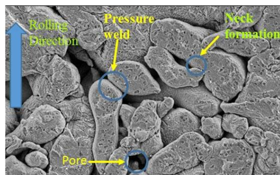
**Figure 10.** SEM-SE image of an aluminium strip surface after being rolled at 0.8 mm and sintered at 580 °C.
