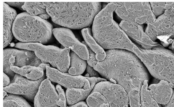
**Figure 9.** SEM-SE image of an aluminium strip surface after being rolled at 0.75 mm and sintered at 580 °C.
