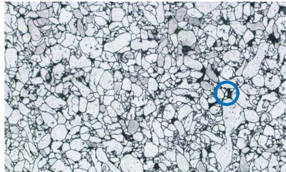
**Figure 5.** Optical image of DPR aluminium strip sintered at 550 °C (pores depicted black, one is exemplarily marked by blue circle).
