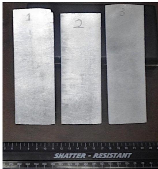
**Figure 2.** Trimmed green aluminium strips produced by DPR process.
