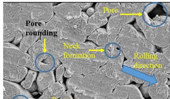
**Figure 13.** SEM-SE image of an aluminium strip surface after being rolled at 0.8 mm and sintered at 580 °C, then re-rolled at 0.75 mm roll gap then re-sintered at 580 °C.
