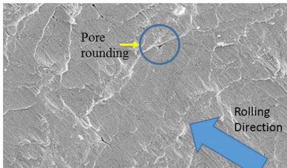
**Figure 11.** SEM-SE image of an aluminium strip surface after being rolled at 0.7 mm and sintered at 580 °C, then re-rolled at 0.65 mm roll gap then re-sintered at 580 °C.
