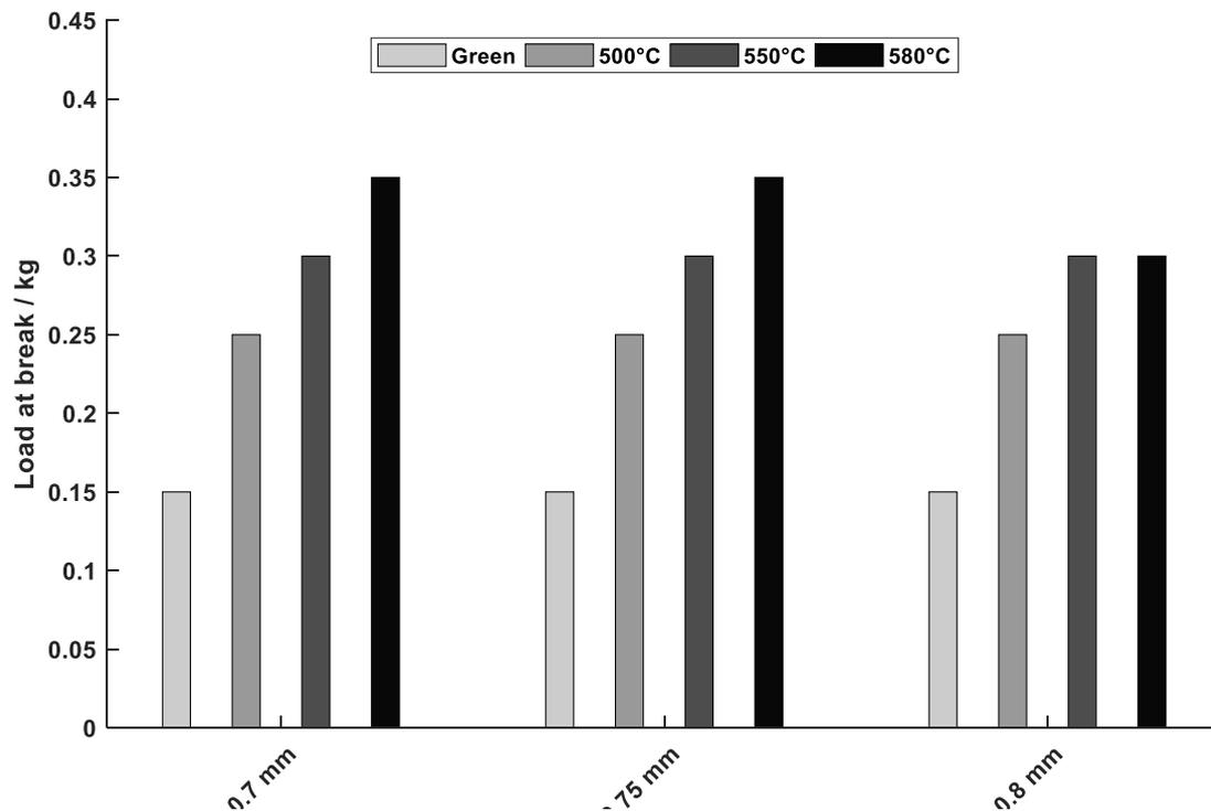
**Figure 15.** Bar graph representing aluminium strip maximum load at failure.
