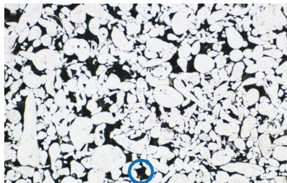
**Figure 3.** Optical image of a green DPR aluminium strip (pores depicted black, one is exemplarily marked by blue circle).
