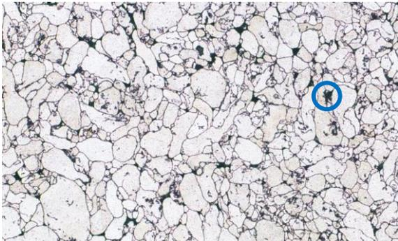
**Figure 6.** Optical image of DPR aluminium strip sintered at 580 °C (pores depicted black, one is exemplarily marked by blue circle).
