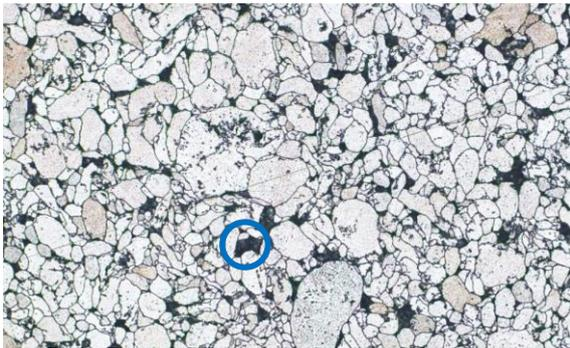
**Figure 4.** Optical image of DPR aluminium strip sintered at 500 °C (pores depicted black, one exemplarily marked by blue circle).
