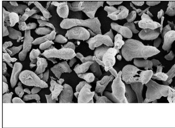
**Figure 1.** SEM-SE image showing the morphology of the aluminium powder.
