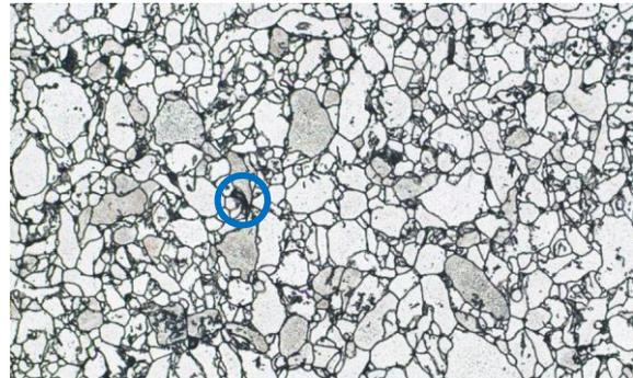
**Figure 7.** Optical image of DPR aluminium strip sintered at 580 °C, rolled at 0.7 mm roll gap and re-sintered at 580 °C (pores depicted black, one exemplarily marked by blue circle).
