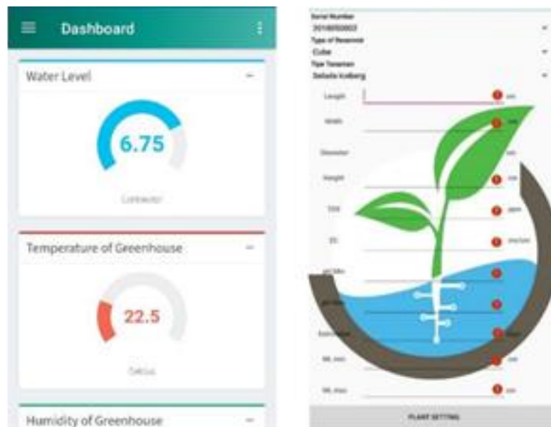
Figure 5. Monitoring and setting threshold levels of nutrient solutions on Android.
