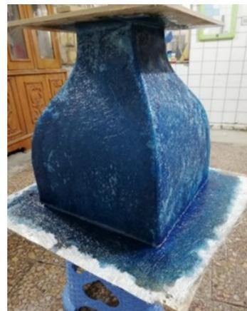
**Figure 12.** The fiberglass model for the selected contraction section.
