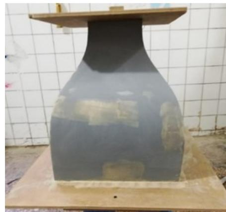
**Figure 11.** Wooden model for the selected contraction section.
