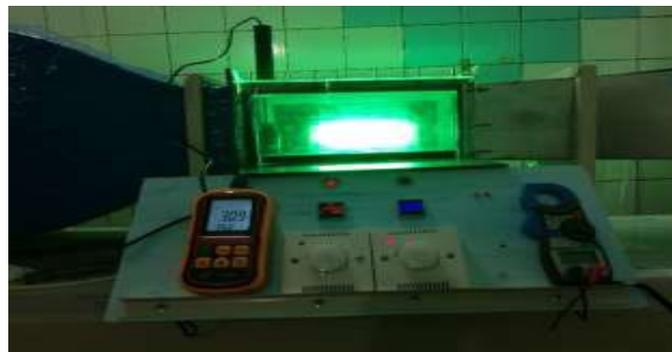
**Figure 14.** Smoke tunnel calibration with an anemometer.
