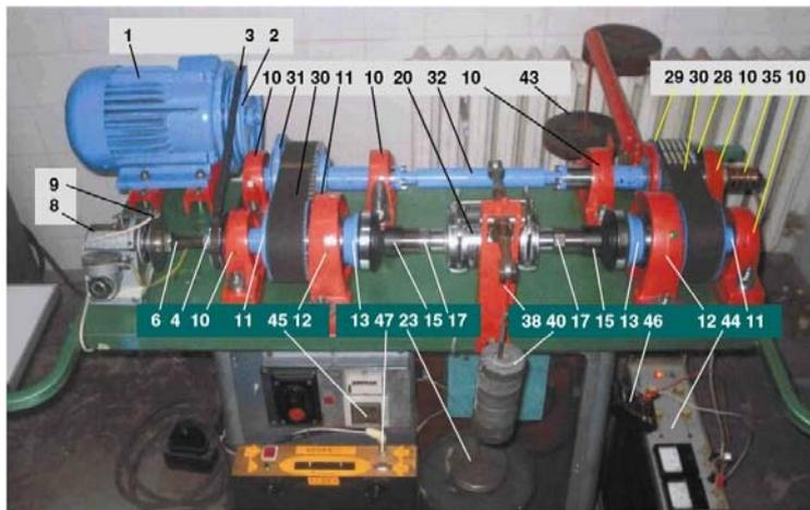
Figure 2. multi-axial fatigue testing machine [17].
