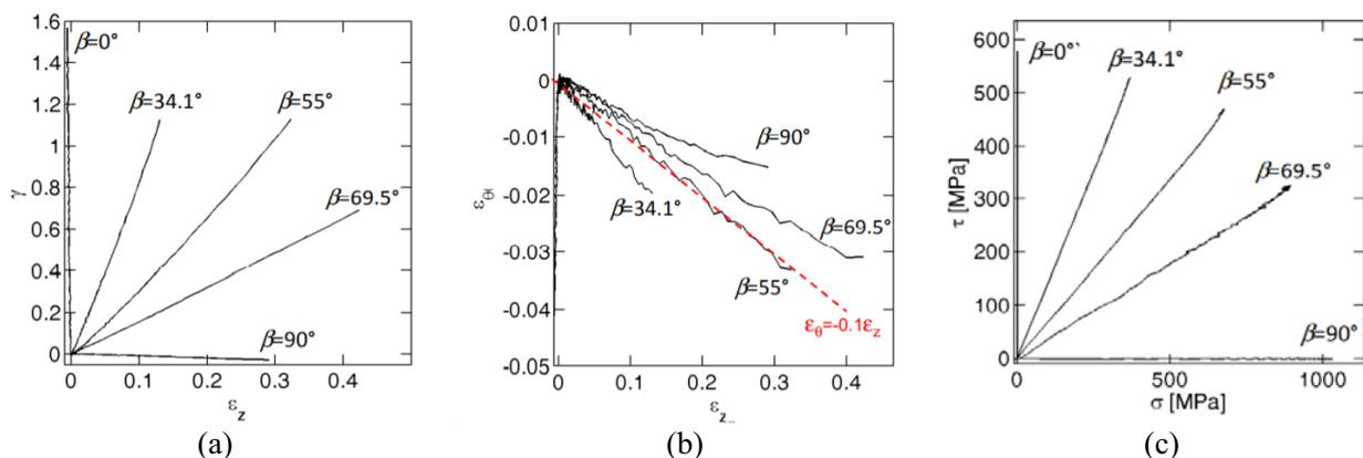
Figure 8. (a) nominal shear vs axial strain loading, (b) nominal peripheral and axial strain loading, (c) means true shear versus true normal stress loading [19].
