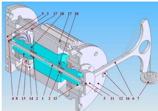
Figure 3. Multi-axial fatigue device [17].
