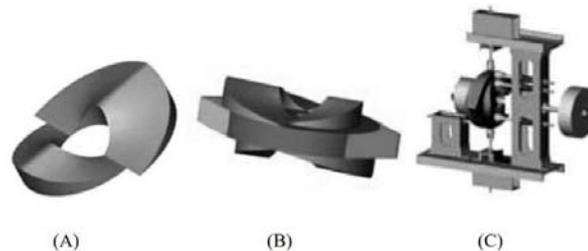
**Figure 6.** Experimental setup (A) bending cams (B) Torsion cams (C) cams-disc and flywheel work mechanism [20].
