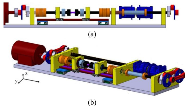
**Figure 4.** Design of the test rig (a) side view and (b) isometric view [18]
