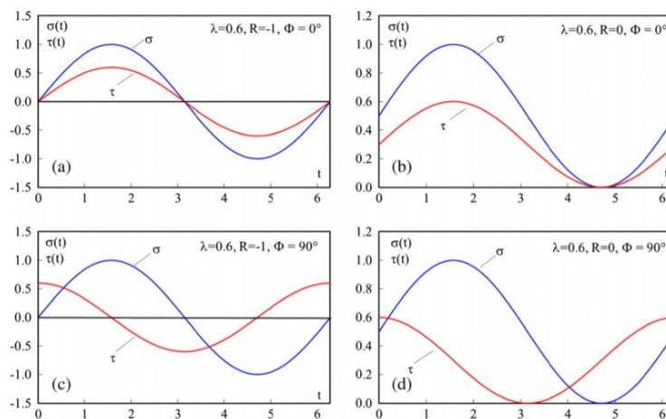
**Figure 9.** Wave forms for all one of multi-axial loading pattern. (a) (b) in phase, and (c) (d) out-of-phase [28].
