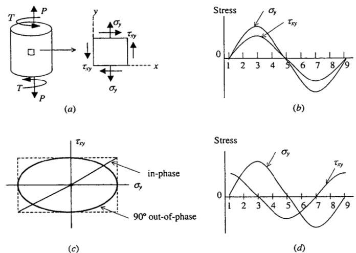
**Figure 1.** Diagram of proportional and nonproportional loading. (a) Axial-torsion loading. (b) In-phase axial loading. (c) Loading path for proportional and nonproportional cases. (d) Out-of-phase axial loading [5].
