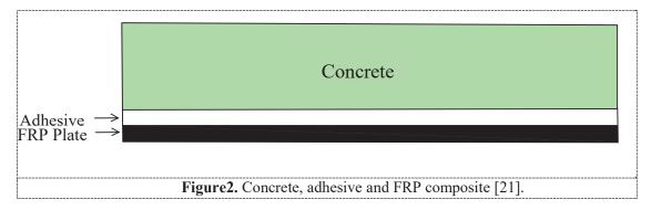
[35] demonstrated that to emphasize the advancement of composite action of the continuous bond among concrete and FRP has been accomplished by adhesives. As the element is in wet conditions these adhesives should not be applied as it could weaken or have negative effects. At the same line [36] reported that environmental conditions like temperature utmost, contacting directly with rain or dust could accelerate or
