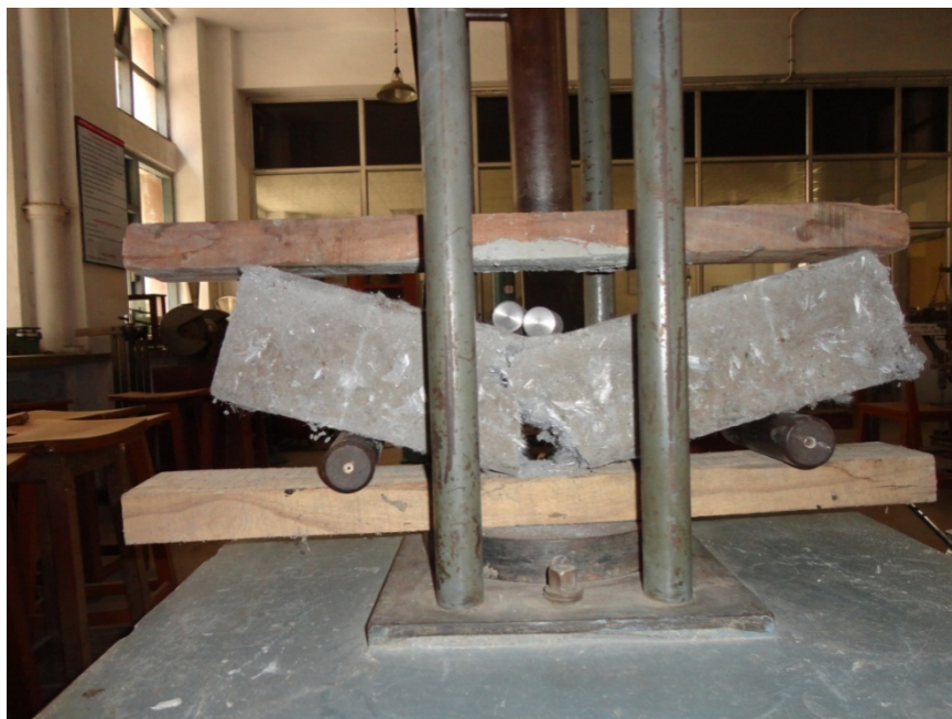
Photograph 1 Typical failure pattern under 2 pt. loading
