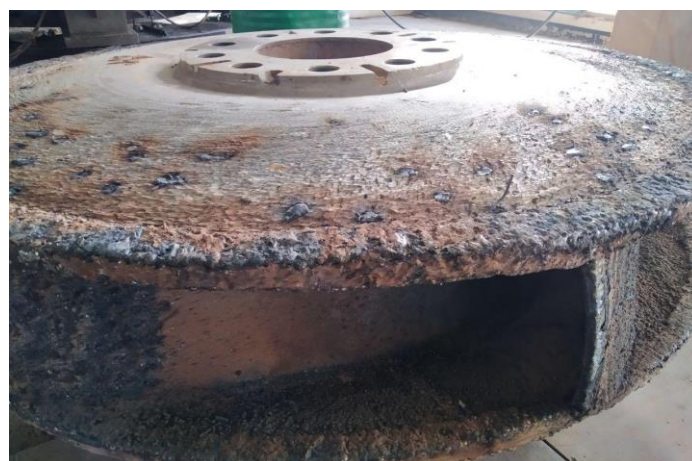
Figure 1. Wear of the impeller of the pumping station Amubukhara 2.
