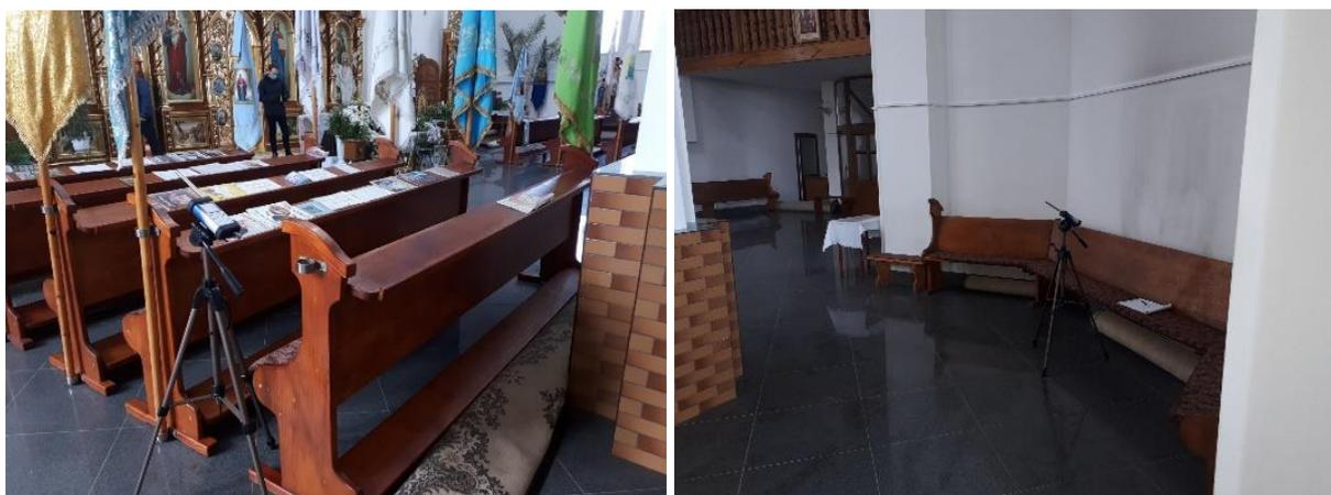
**Figure 4.** Reverberation time measurement.
