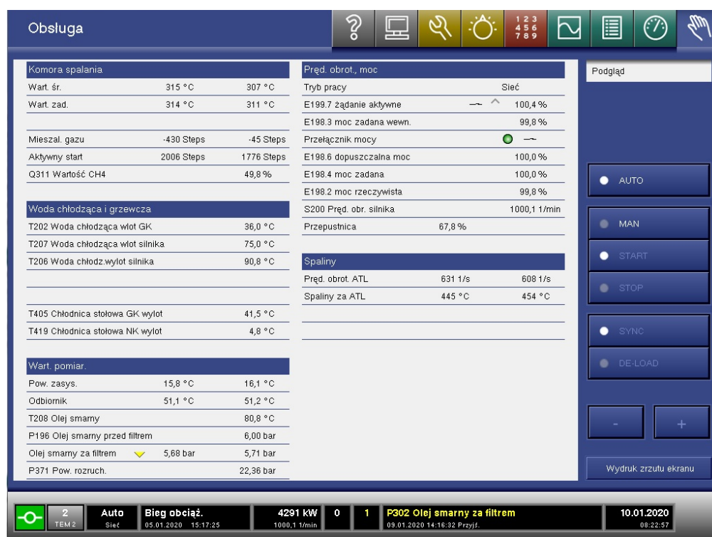
Figure 2. The real cogeneration aggregate control display.
