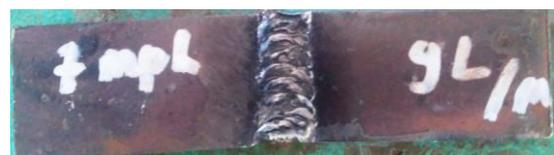
**Figure 9.** Macro structure of weld metal at gas discharge 9 L/min with wind speed of 7 mph.
