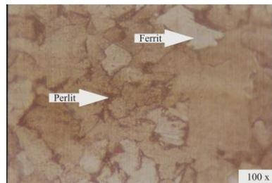
**Figure 4.** Microstructure of weld metal at gas discharge 9 L/min with wind speed of 3 mph.
