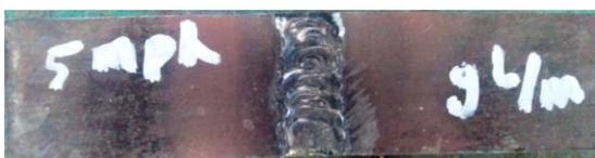
**Figure 8.** Macro structure of weld metal at gas discharge 9 L/min with wind speed of 5 mph.
