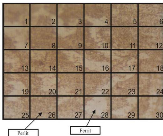
**Figure 3.** The calculation of ferrite and pearlite at 3 mph wind speed with a discharge rate of 9 L/min on HAZ
