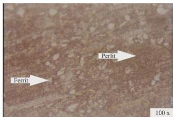
**Figure 5.** Microstructure of weld metal at gas discharge 9 L/min with wind speed of 5 mph.
