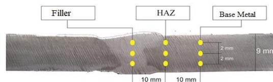
**Figure 1.** The classification area of temperature cycle effect on TIG welding process.
