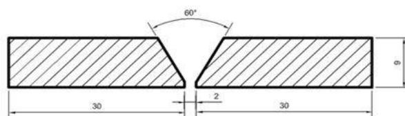
**Figure 2.** The dimension of TIG Specimen test.
