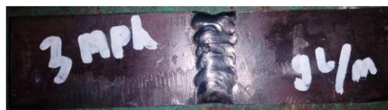
**Figure 7.** Macro structure of weld metal at gas discharge 9 L/min with wind speed of 3 mph.
