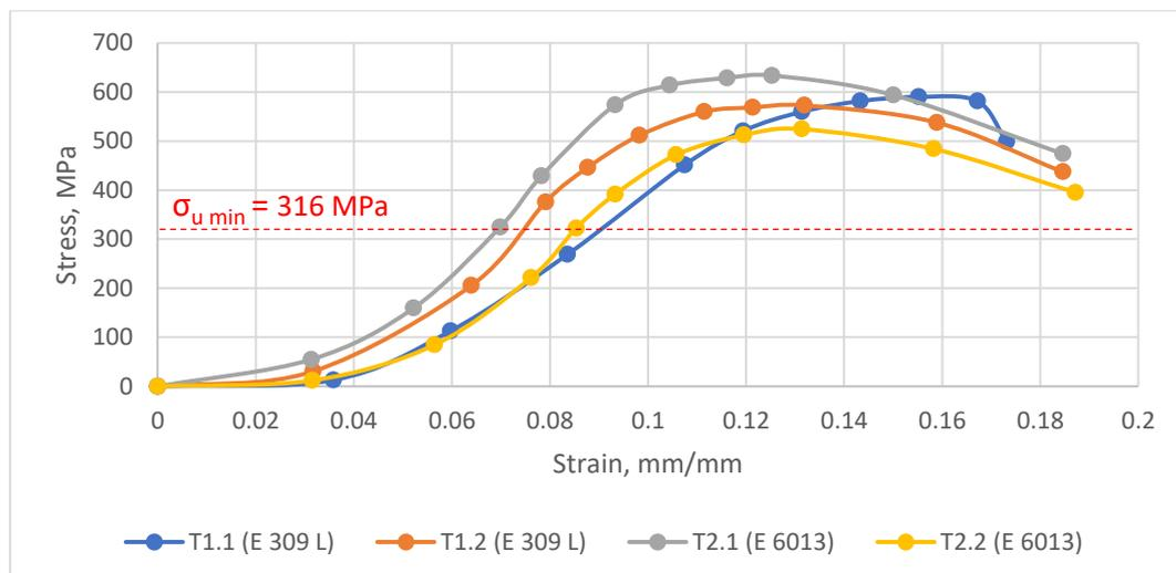
**Figure 2.** Stress – Strain engineering graph for each specimen tensile test result.
