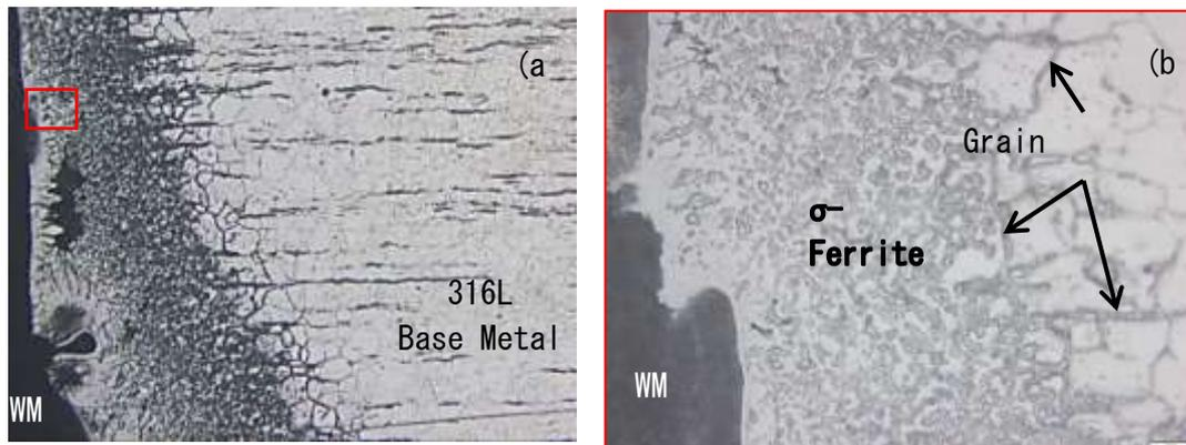
**Figure 7.** Microstructure of E6013 weld metal to AISI 316L base metal magnification (a) 100 x (b) 500 x
