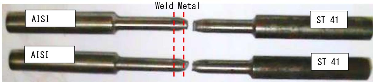
**Figure 3.** Tensile test specimen after tensile force applied.
