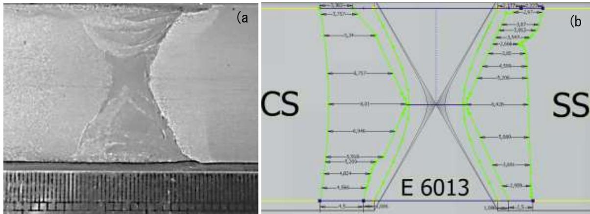
**Figure 5.** Macrostructure of joint ST41 and AISI 316L with E6013 rod (a) raw image; (b) re-measuring groove and dilution.
