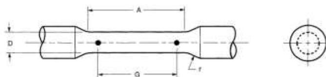
**Figure 1.** Round bar test specimen illustration
