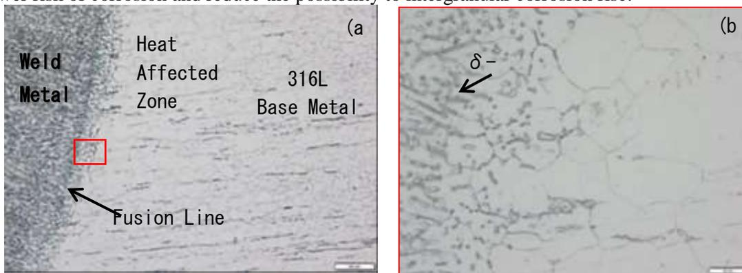
**Figure 6.** Microstructure of E309L weld metal to AISI 316L base metal magnification (a) 100 x (b) 500 x
