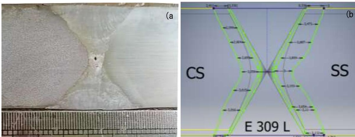
**Figure 4.** Macrostructure of joint ST41 and AISI 316L with 309L rod (a) raw image; (b) re-measuring groove and dilution.
