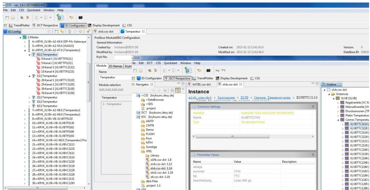
**Figure 2:** Screenshot of the PROFIBUS and PV configuration tools in Control System Studio (CSS).
