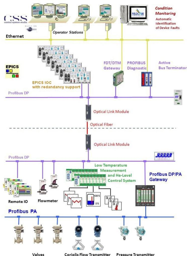
**Figure 1:** The EPICS based cryogenic control system uses distributed I/O. The selected field bus is PROFIBUS DP. All valves' positioners and most sensors are connected through PROFIBUS PA which also provides power. The in house developed low temperature measurement system is attached to PROFIBUS as well. Ethernet to PROFIBUS gateways provide access to the PROFIBUS components for the condition monitoring application.
