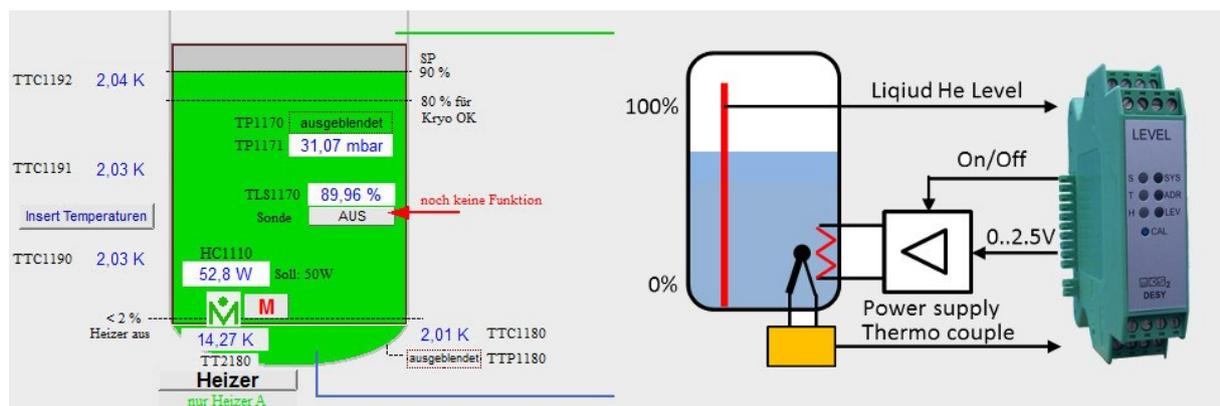
**Figure 6:** Typical installation of Helium vessel with LHe level sensor and heater
