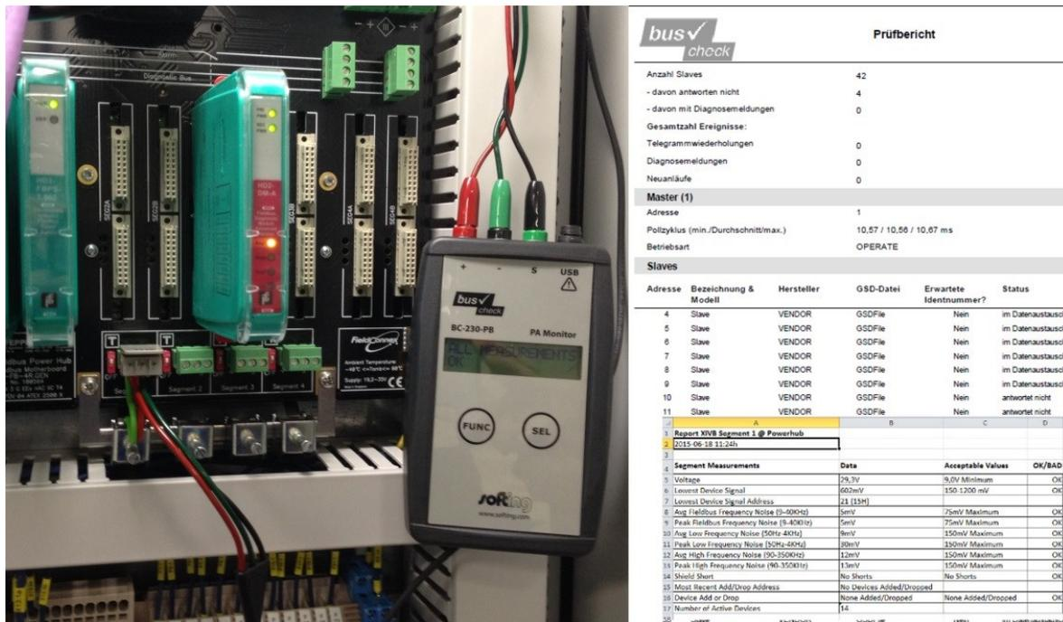
Figure 4: PROFIBUS PA segment checker and test reports
