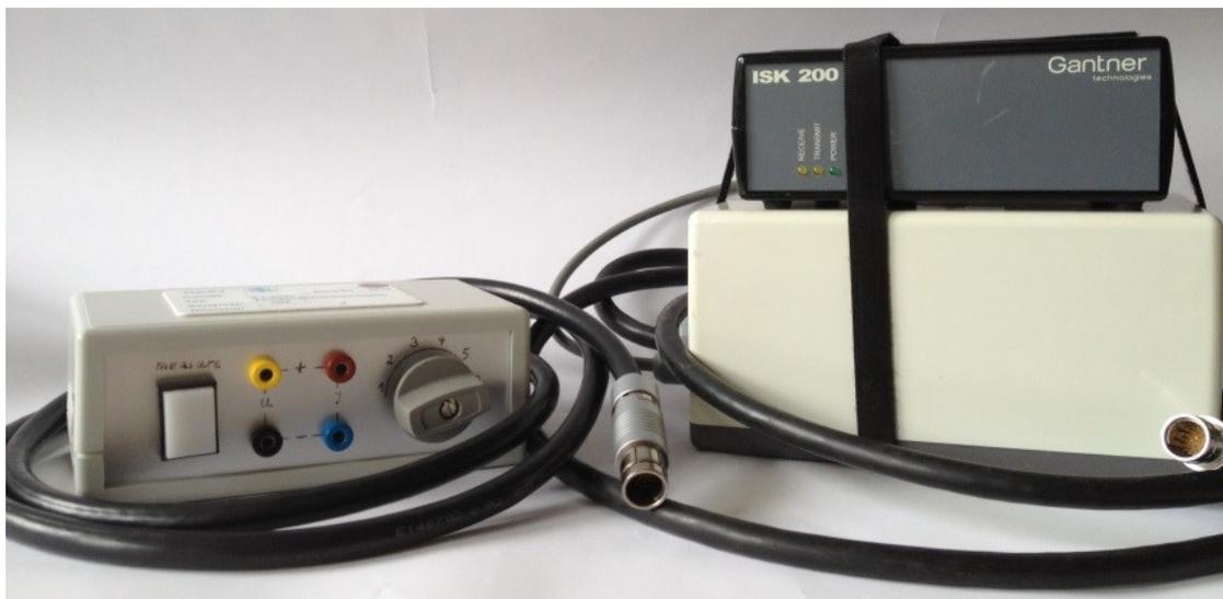
**Figure 7:** Test boxes for temperature measurements. Left side the simple box and on the right side the Gantner box.
