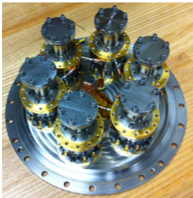
Figure 5. Model heat switches used to test the new flange design. This design allows the screws that mate the heat switch to other components in the system to not compress the indium seal (see also Figure 3). For the test, the switches are bolted to the end cap of a vacuum vessel and a thermometer is added to track the temperature of the cap. The assembly is then sealed to the vacuum vessel using an indium wire and cooled to 77 K slowly while measuring the presence of helium in the vessel interior.
