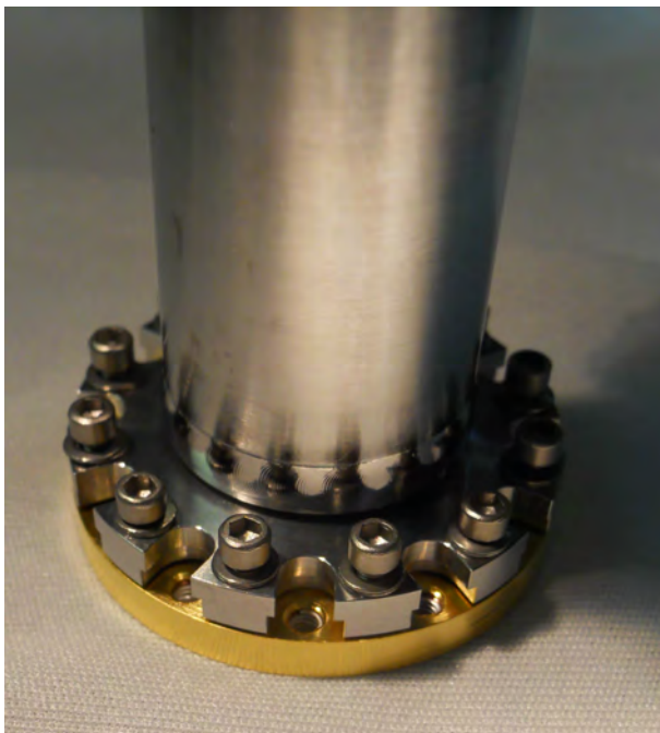
Figure 3. An indium seal is compressed between the flange brazed to the outer shell and the conducting fins inserted to the interior. The crenellated design of the flange allows the bolts that compress the indium seal to be taken out of the joint used to join the switch to other components. Since the heads of those bolts fit inside the machined opening in the flange and don't compress the indium seal, integrating or removing the switch from an assembly does not disturb the indium increasing its reliability.
