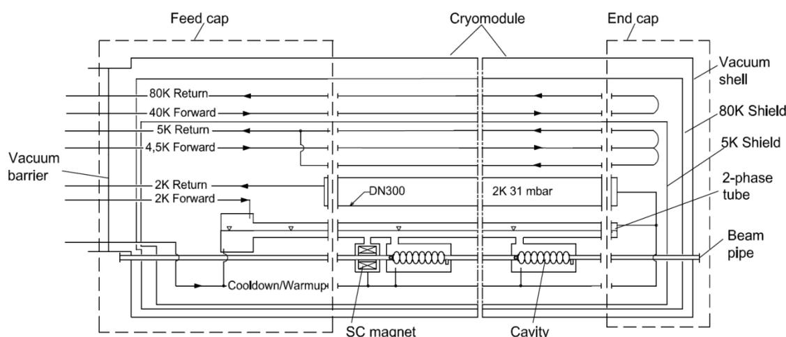
**Figure 3.** AMTF simplified scheme of Feed cap, End cap and Cryomodule.
