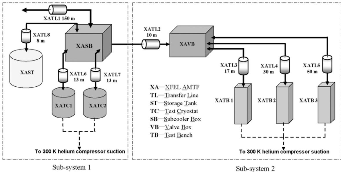
**Figure 1.** Schematic view of AMTF cryogenic infrastructure
