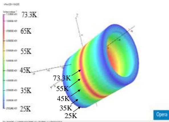
**Figure 5.** Post-quench transient thermal mapping after 1 s simulated for the NbTi magnet using OPERA (Vector Field) FEA code.
