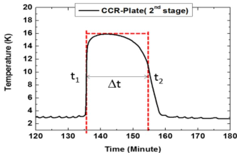
**Figure 7.** Post-quench temperature profile of the CCR-plate of the 2<sup>nd</sup> stage of the cryocooler.
