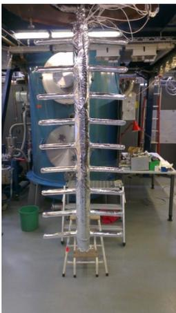
**Figure 5a.** Cylinder (B) with 12 layers MLI of RUAG
