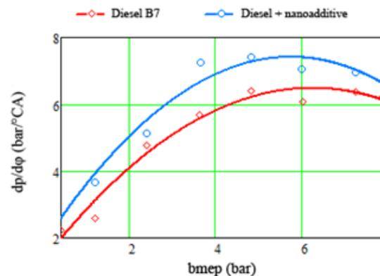
**Figure 6.** First derivative of in-cylinder pressure  $dp/d\phi$  vs brake mean effective pressure  $bme_p$ .
