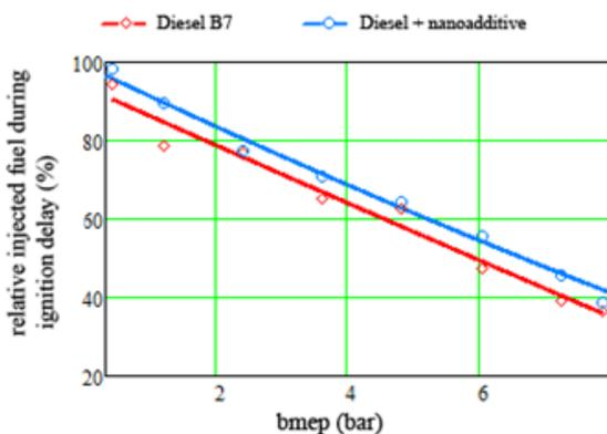
**Figure 5.** Relative quantity of injected fuel during ignition delay vs brake mean effective pressure  $bme_p$ .
