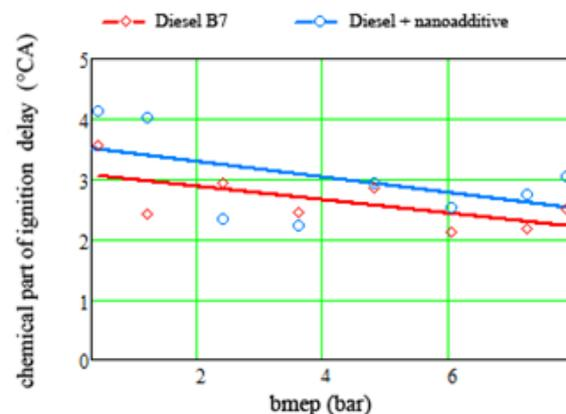
**Figure 2.** Duration of chemical part of ignition delay vs brake mean effective pressure *bmeep*.
