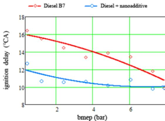
**Figure 3.** Ignition delay, determined by line of heat release rate, vs brake mean effective pressure  $bme_p$ .
