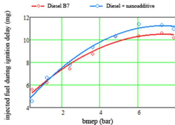
**Figure 4.** Quantity of injected fuel during ignition delay in mg vs brake mean effective pressure  $bme_p$ .
