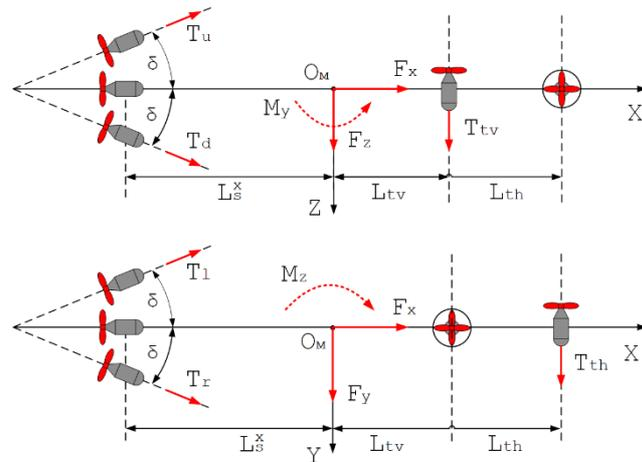
**Figure 2.** The principal structure of the AUV “MMT-300” propulsion system.
