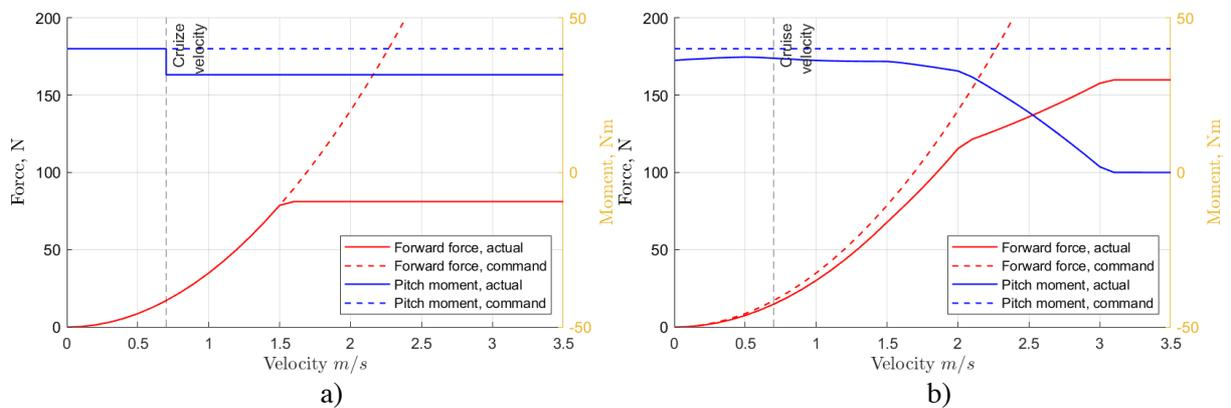
**Figure 4.** Control allocation with the adaptive optimal allocation method based on the fixed point theorem. There are thrust (a) and forces (b) allocation in the left and right image, respectively.
