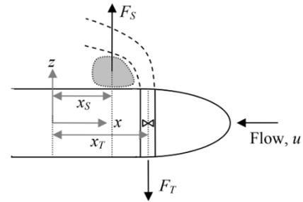
**Figure 1.** Propulsion jet of through-body thruster.
