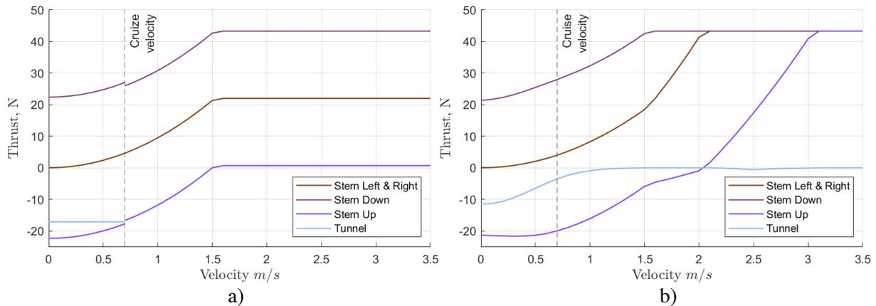
**Figure 3.** Control allocation with the prioritized direct allocation method. There are thrust (a) and forces (b) allocation in the left and right image, respectively.
