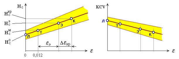
L - the state of the sheet, T - the state of the new pipe, E - in a state of operation for 50 years, K - critical state when KCV reaches the lower allowable value.
