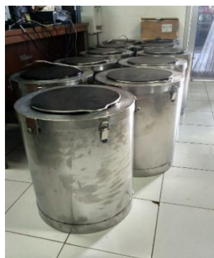
Figure 4. Stainless steel canister for \text{U}_3\text{O}_8 package as the final waste form of the RFW from ^{99}\text{Mo} production.
