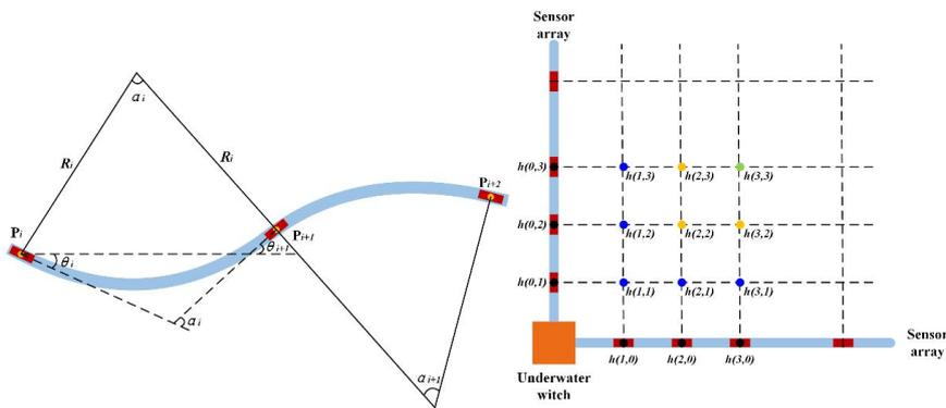
**Figure 3.** The arc model (The blue one is the sensor array, while the red one is the MEMS sensor). **Figure 4.** Interpolation schematic.
