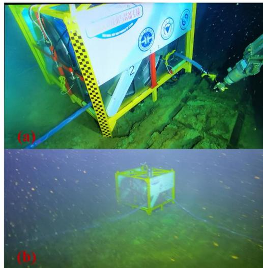
**Figure 8.** (a) ROV's Manipulator pull out the sensor array; (b) Sensor array deployment.
