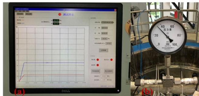
**Figure 6.** (a) Pressure curve; (b) Pressure indicator.
