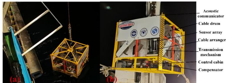
**Figure 7.** (a) Underwater winch hoisting; (b) Underwater winch.
