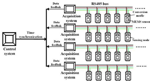
**Figure 2.** The acquisition and control system.
