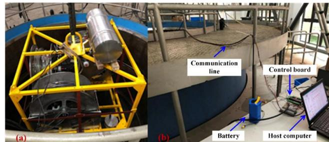
**Figure 5.** (a) Underwater winch hoisting; (b) connection between host computer and control board.
