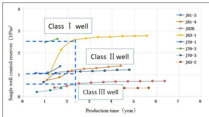
**Figure 8.** Change curves of controlled reserves in different production stages
