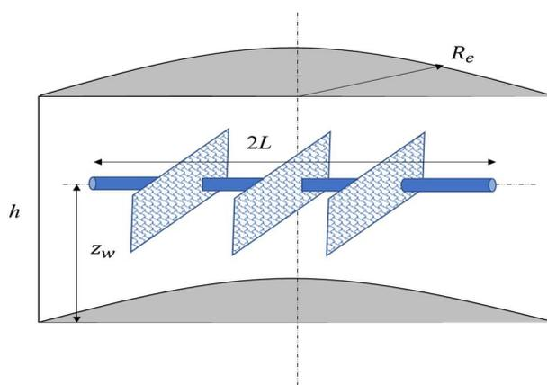
**Figure 1.** Schematic diagram of staged fracturing for tight sandstone gas reservoirs
