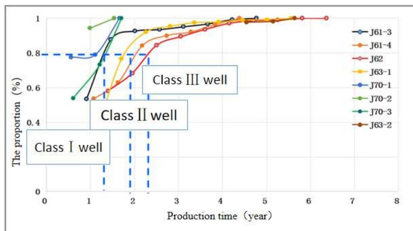
**Figure 9.** Ratio curves of single well-controlled reserves to final recoverable reserves at different production stages
