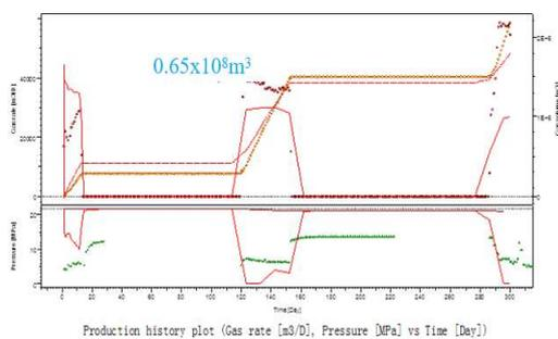
**Figure 3.** Fitting analysis curve of Jiao 61-3 well production history (1 year)
