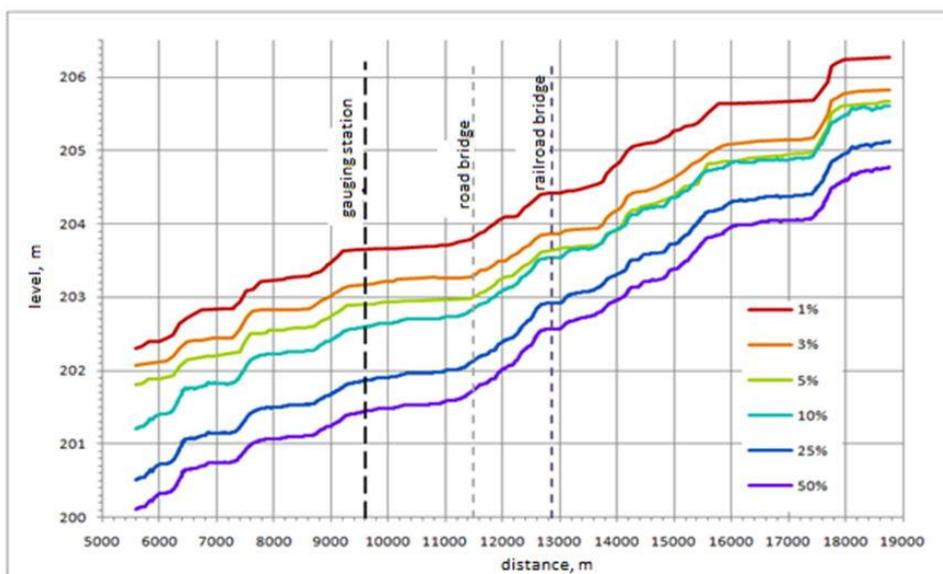
**Figure 6.** Longitudinal profile of the water surface of the river Kahn with high water and high flows 1%, 3%, 5%, 10%, 25% and 50%.
