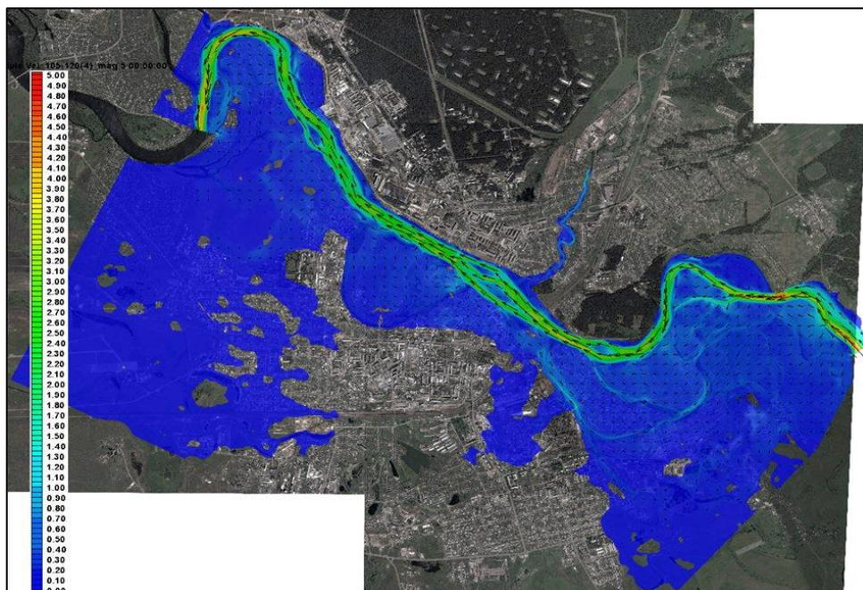
**Figure 5.** The field of velocities in the flooding zone of the territories adjacent to the rivers Kan and Ilanka within the city of Kansk flooded during high water and high flows 1% of availability.
