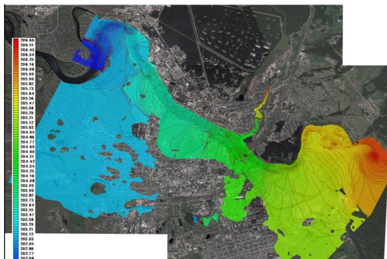
**Figure 3.** Levels of the free surface of the water in the flooding zone of the territories adjacent to the rivers Kan and Ilanka within the town of Kansk, flooded during high water and high flows 1% of availability.
