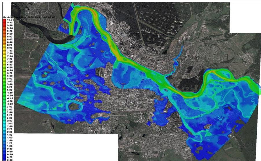
**Figure 4.** Water depth in the flooding zone of the territories adjacent to the rivers Kan and Ilanka within the city of Kansk, flooded during high water and high flows 1% of availability.
