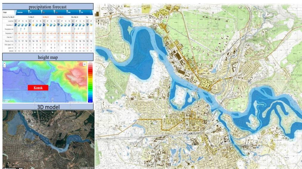
**Figure 8.** Model of flood on the Kan River near Kansk.
