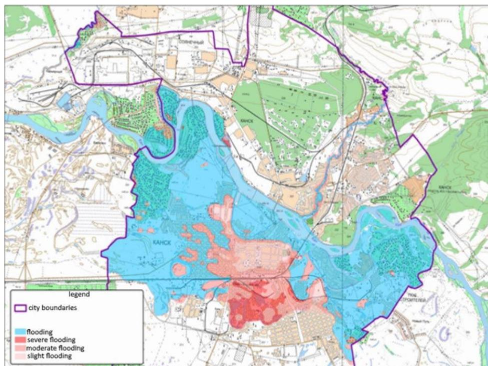
**Figure 7.** Graphic representation of the boundaries of areas of flooding of territories during high water and high flow of 1% of the rivers Kan, Ilanka, Kurysh within Kansk.
