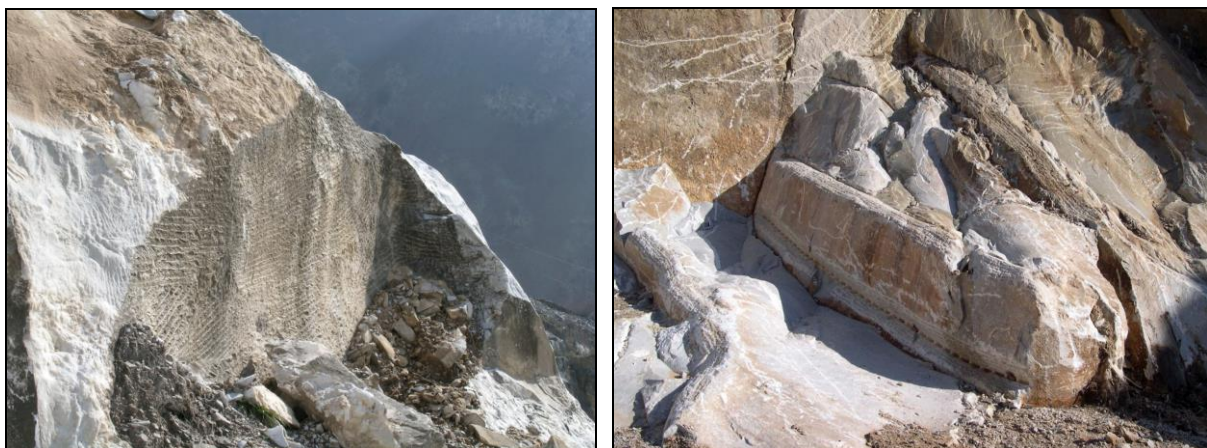
Figure 4. Roman cuts: left – festooned cut ( caesura ) along the contro in large fracture spaced rock-mass; right – base tiled-cut in fractured rock along the verso .
