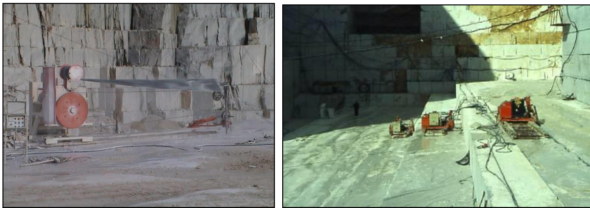
Figure 9. Left) diamond-wire cutting machine; right) battery of toothed chain saws.
