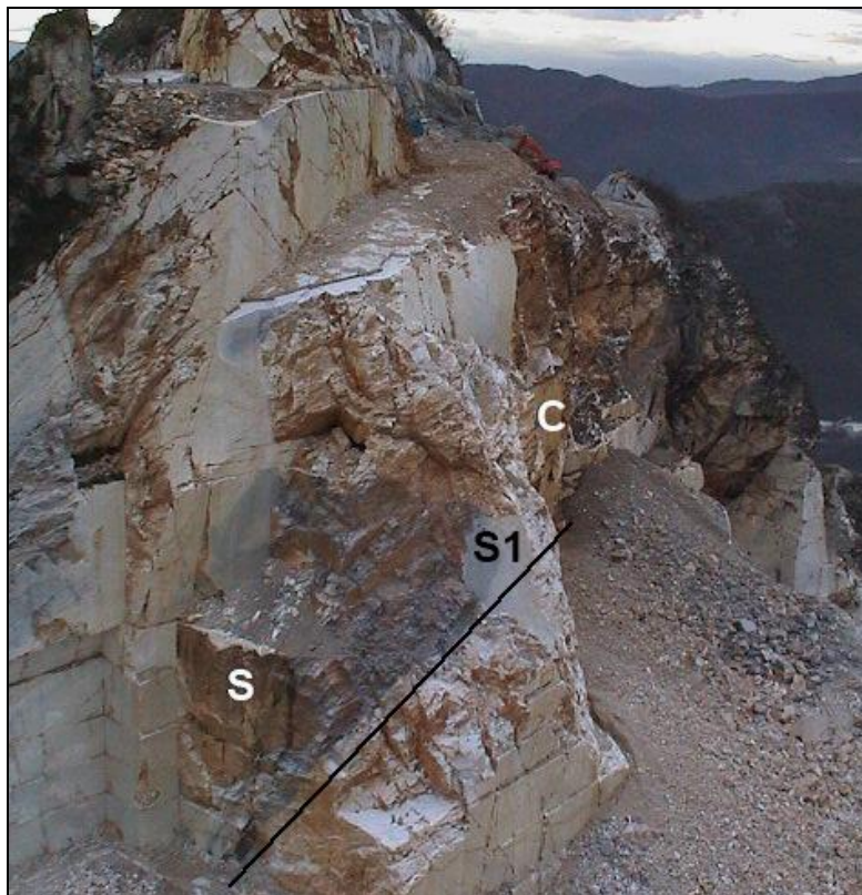
Figure 1. Reciprocal relationship among the Verso (S1) main schistosity and the two fracture systems: Secondo (S) and Contro (C).
