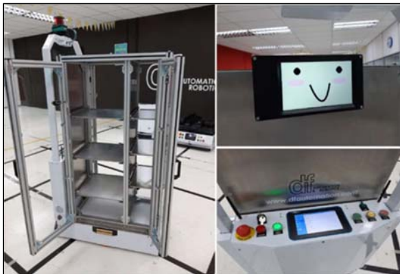
Figure 5. Left picture: Customizable compartment shelves. Right Top picture: The LCD screen displays an animated friendly face. Bottom Right Picture: Graphical User Interface (GUI).
