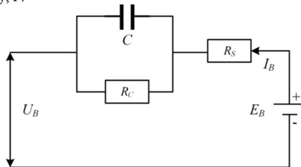
**Figure 2.** Thevenin's equivalent circuit of battery energy storage system.
