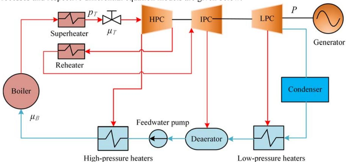
**Figure 1.** Diagram of boiler-turbine system for a coal-fired power unit.
