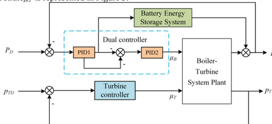
**Figure 3.** Diagram of the improved strategy for the boiler-turbine system.
