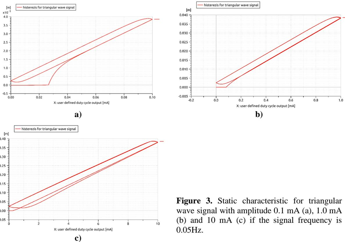
**Figure 3.** Static characteristic for triangular wave signal with amplitude 0.1 mA (a), 1.0 mA (b) and 10 mA (c) if the signal frequency is 0.05Hz.
