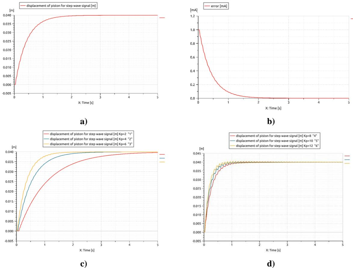
**Figure 9.** Influence of  $K_p$  coefficient of the P controller for step signal with amplitude of 1 mA: a) rod displacement, b) the error, c) and d) the dynamics for different  $K_p$  values.
