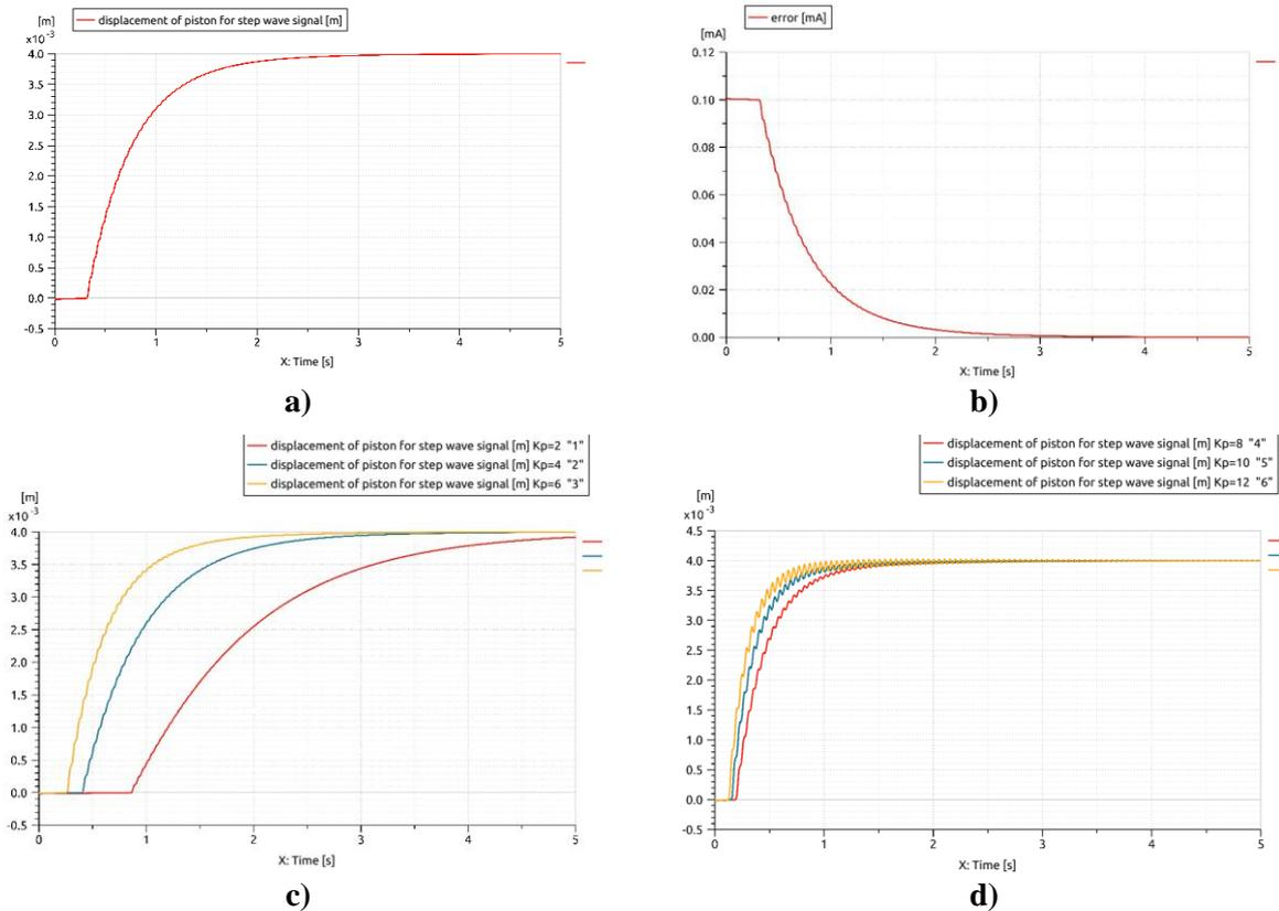
**Figure 8.** Influence of  $K_p$  coefficient of the P controller for step signal with amplitude of 0.1 mA: a) rod displacement, b) the error, c) and d) the dynamics for different  $K_p$  values.
