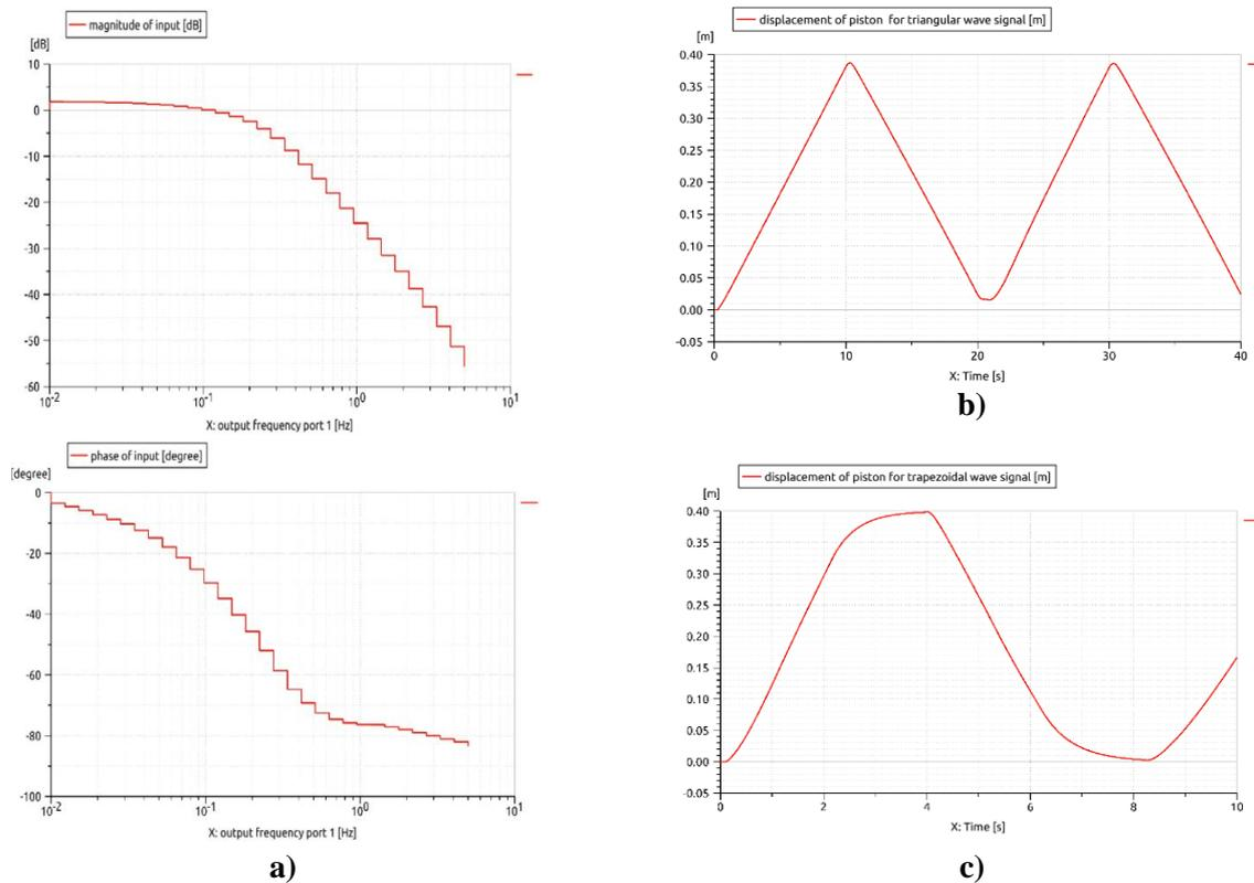
**Figure 5.** Dynamic characteristic: a) Bode diagram; b) rod displacement at triangular wave input; c) rod displacement at trapezoidal wave signal.
