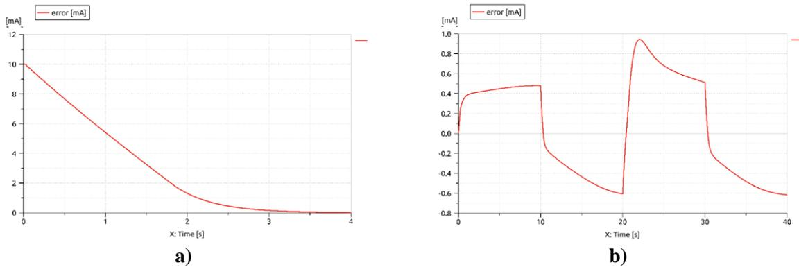
**Figure 4.** The error in rod displacement to different inputs: b) 10mA step input, c) 1mA triangular wave
