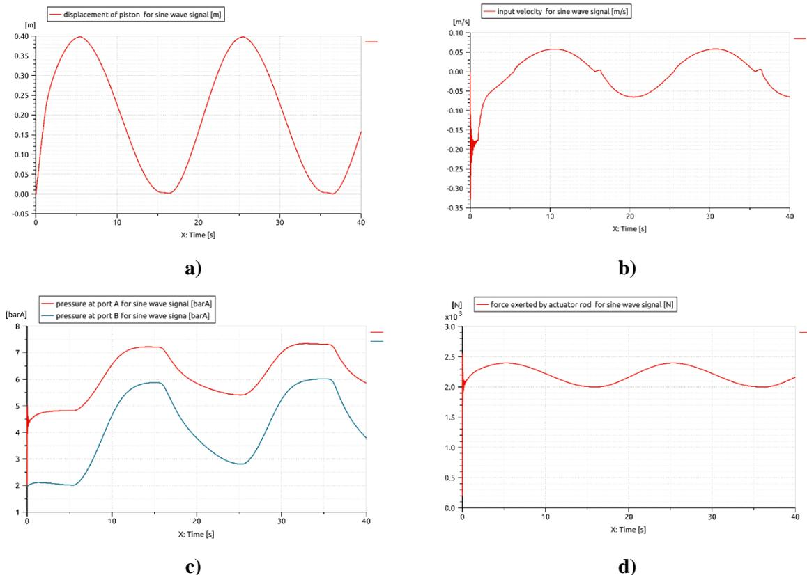
**Figure 7.** Dynamic behaviour to sine wave signal with 10mA amplitude and 50Hz frequency: a) rod displacement, b) rod velocity, c) pressures in cylinder chambers, d) force at the rod.
