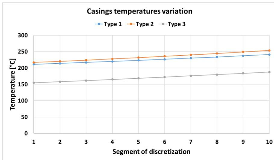
**Figure. 10** Wall temperatures of the metal casings ( $T_{met}$ )
