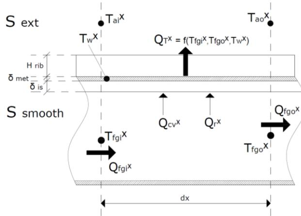
**Figure. 3** A BC discretization segment with parameters and heat fluxes
