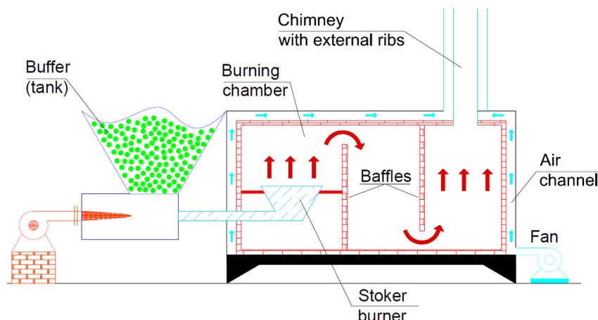
**Figure. 4** Simplified combustion chamber scheme with the Stocker burner, two baffles and a metallic casing
