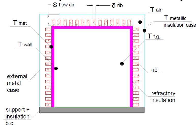
**Figure. 6** BC front section with geometrical elements and parameters
