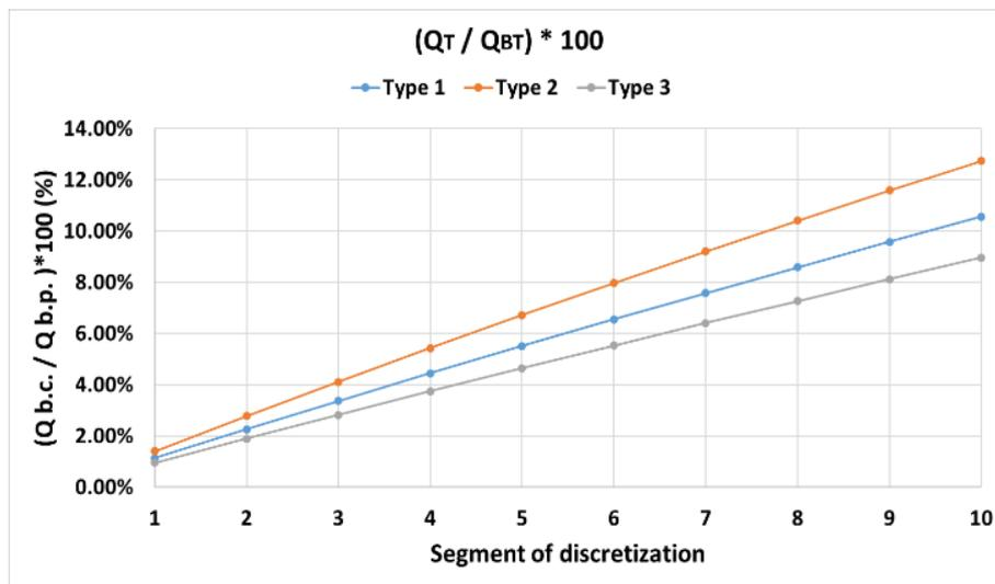
**Figure. 12** Percentage of total heat flux, radiation and convection ( $Q_T$ ), in regards to the thermal power of the burner ( $Q_{BP}$ );  $[(Q_T / Q_{BP}) * 100]$
