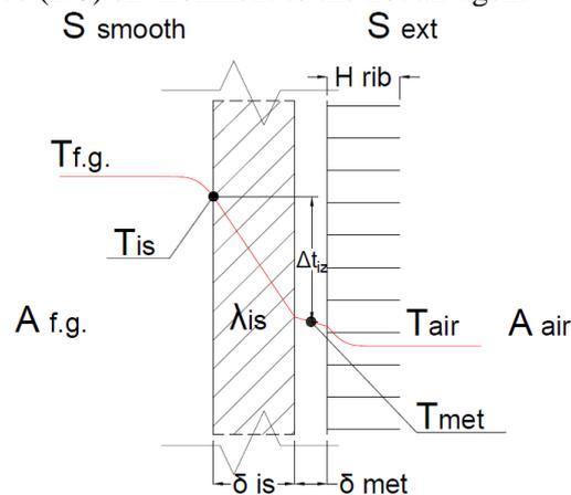
**Figure 1** Schematic temperature variation and heat transfer parameters between two environments
