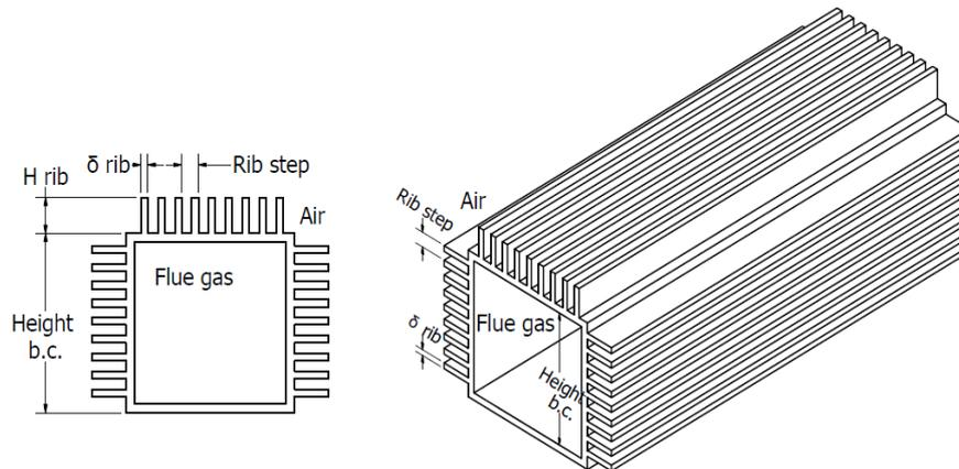
**Figure. 5** BC geometry: front section and 3D isometric view, without the metallic case
